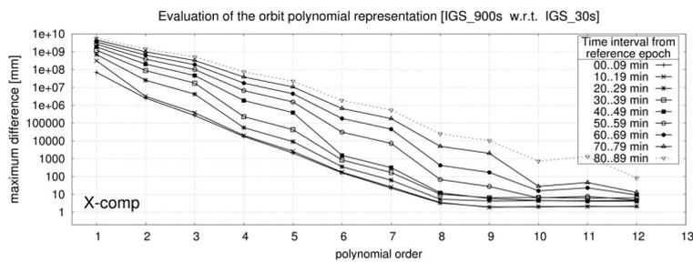
**Fig. 9** Polynomial degree test with respect to the validity interval – IGS orbits sampled at 900s intervals were interpolated and compared with respect to the same orbits sampled originally at 30s intervals.
