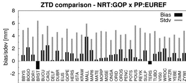
**Fig. 11** The comparison of GOP near real-time ZTDs with EUREF combined ZTD produkt.
