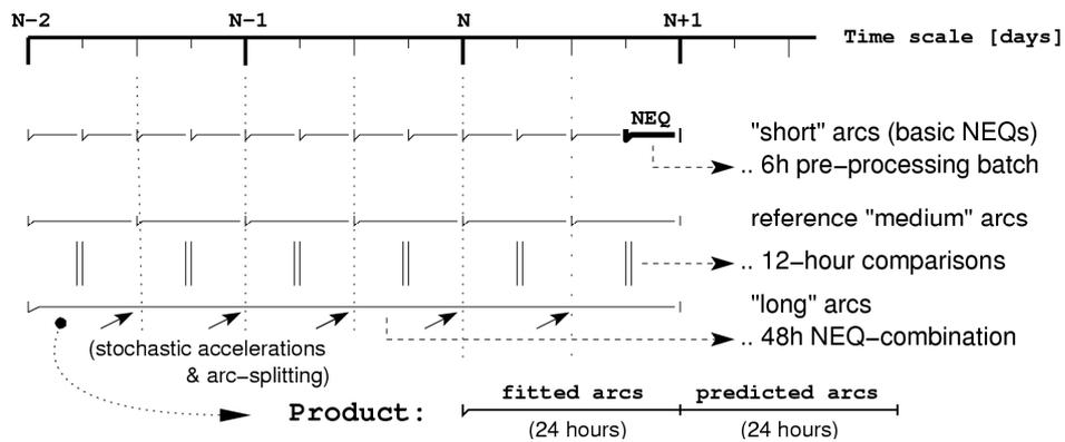
Fig. 2 Chart of the long-arc orbit combination procedure.
