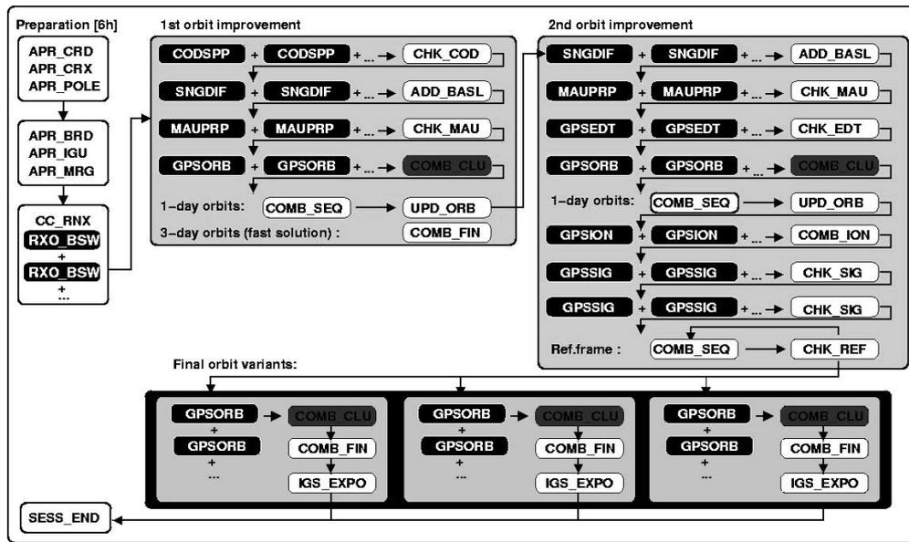
Fig. 1 GOP ultra-rapid orbit processing blocks. Black boxes are processed in parallel.
