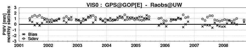
**Fig. 12** Monthly statistics of the GPS and radiosonde PWV comparison (stationVIS0).
