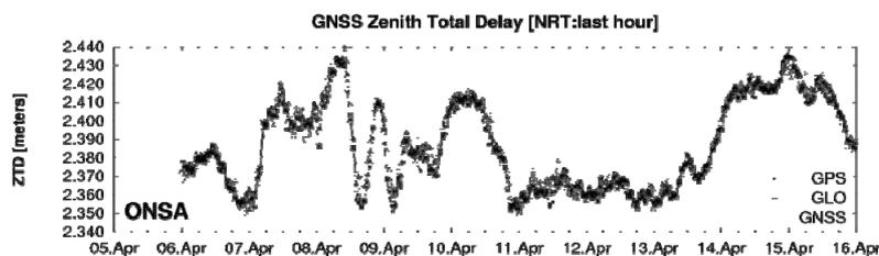
Fig. 13 Time-series for zenith total delay parameters estimated at stations ONSA (Onsala) using GPS, GLONASS or both data.
