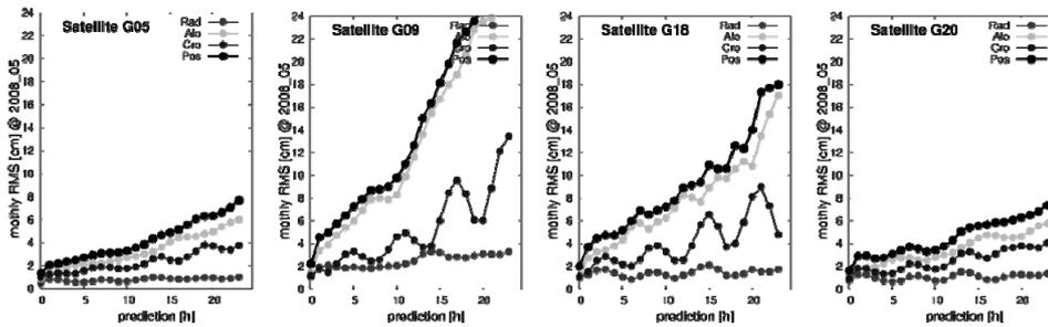
**Fig. 7** Monthly IGS ultra-rapid orbit prediction errors for the satellites G05, G09 (Block IIA) and G18, G20 (Block IIR) plotted with respect to the prediction interval. Satellites G09 and G18 were affected by the eclipsing period, while satellites G05 and G20 were not.
