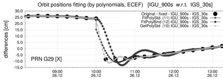
**Fig. 8** Three methods of the polynomials estimation: GetPolyStd (Lagrange form), FitPolyStd (unconditional fitting), FitPolyBind (fitting conditional for the consistency in the coordinates and velocities).
