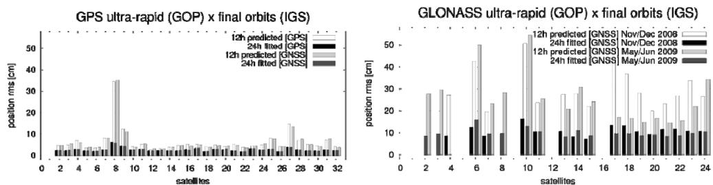
**Fig. 5** The left figure shows the position RMS for GPS satellites from stand-alone GPS and GNSS solution for 12h-predicted and 24h-fitted interval. The right figure shows the position RMS for GLONASS satellites from GNSS solution in two periods.
