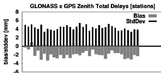
Fig. 14 Inter-comparisons of GLONASS and GPS based ZTDs for all processed stations (x-axis).
