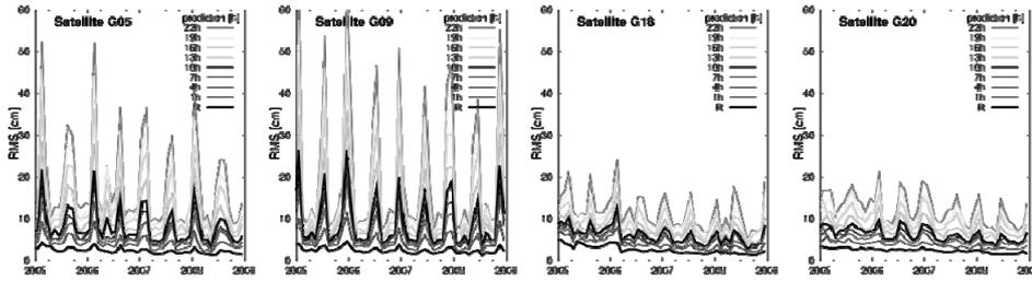
**Fig. 6** The time-series of the satellite G05, G09 (Block IIA) and G18, G20 (Block IIR) IGS ultra-rapid orbit predictions (fit, 1h, 4h, 7h, 10h, 13h, 16h, 19h and 22h) compared to IGS final orbits (monthly average).
