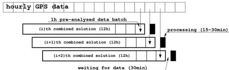
**Fig. 10** Near real-time ZTD estimation scheme – hourly NEQs and 12-hour combination.
