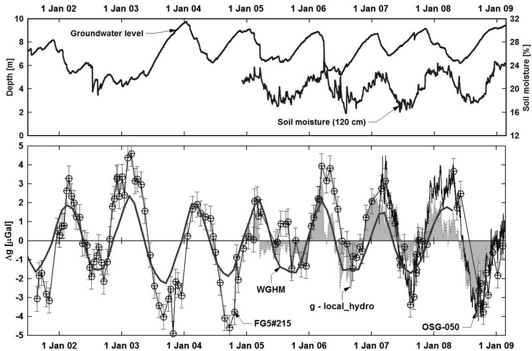
**Fig. 6** Top: Variations of the groundwater level and the soil moisture in the depth of 120 cm. Bottom: Gravity variations at the Pecný station based on the measurement with the FG5#215 and OSG-050. The curve “g-local\_hydro” represents the corrected gravity series for local hydrological effects. The curve WGHM is the effect of the continental water storage variation based on the WGHM data.
