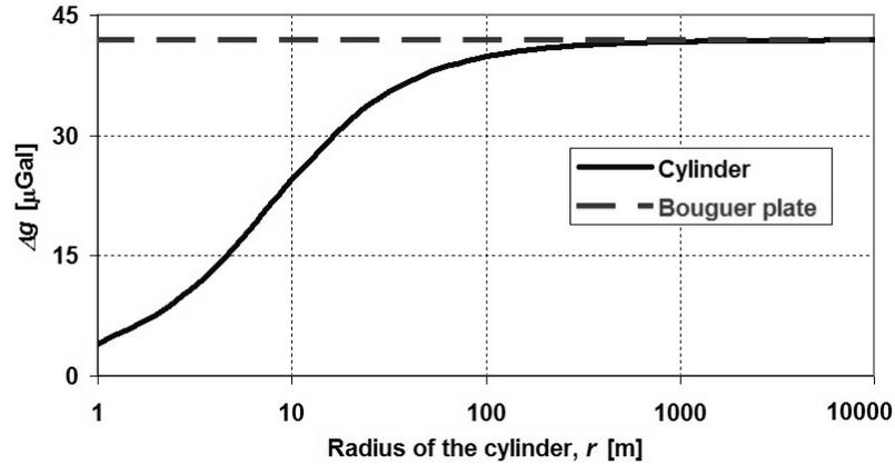
**Fig. 5** Gravity variation caused by the Newtonian attraction of water masses homogeneously distributed within the 10 m thick cylinder with 10% porosity and variable radius.
