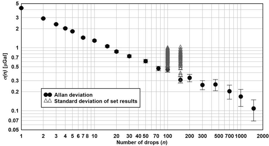
**Fig. 1** The Allan deviation and the standard deviation of the set results computed from the FG5#215 measurements at the Pecný station.
