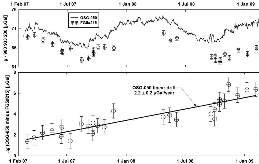
**Fig. 2** Top: Time series of the OSG-050 and the FG5#215 at the Pecny station. Bottom: Differences between SG and AG allow to determine a long-term reproducibility of the FG5#215 (represented by error bars  $0.7 \mu\text{Gal}$ ) and the instrumental drift of the OSG-50 (linear term  $2.2 \mu\text{Gal}/\text{year}$ ).
