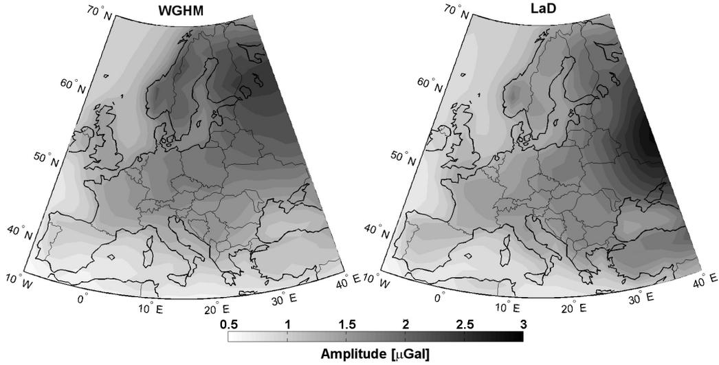
**Fig. 4a** Amplitude of the annual harmonic function which represents the gravity effect caused by continental water storage variations based on the WGHM and LaD models.
