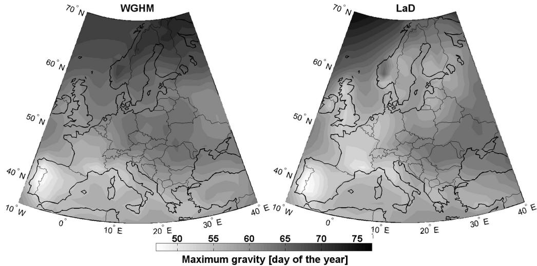
**Fig. 4b** Phase of the annual harmonic function which represents the gravity effect caused by continental water storage variations based on the WGHM and LaD models.
