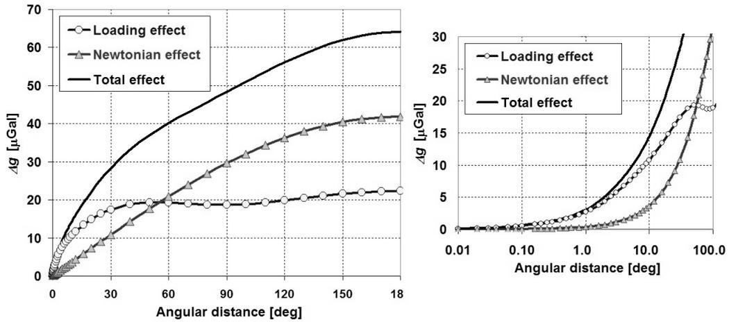
**Fig. 3** Effect on gravity (loading part, Newtonian part and the total effect) caused by a centered homogeneous shell of water (of angular distance) and thickness of 1 m. The right figure is depicted by logarithmic scale in the horizontal axis for better interpretations of the effect for lower angular distances.
