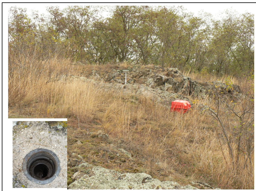
Fig. 8 Geodetic stabilization of GPS point NAHO – Načeratická hora (1993 – ČVUT), part of former geodynamical network Morava. Measured during campaign in October 2009.
