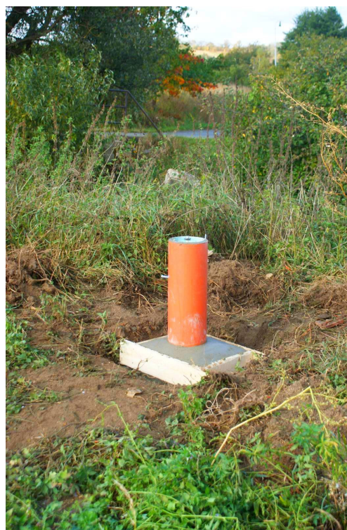
Fig. 6 Deeply stabilized GPS point at Tetčice locality near railway station
