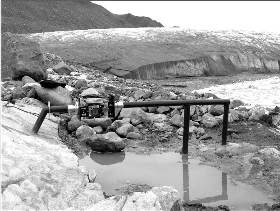
**Fig. 1** An example of the TM71 extensometric gauge installed in Hornsund, Spitsbergen (Photo: T. Nýdl).
