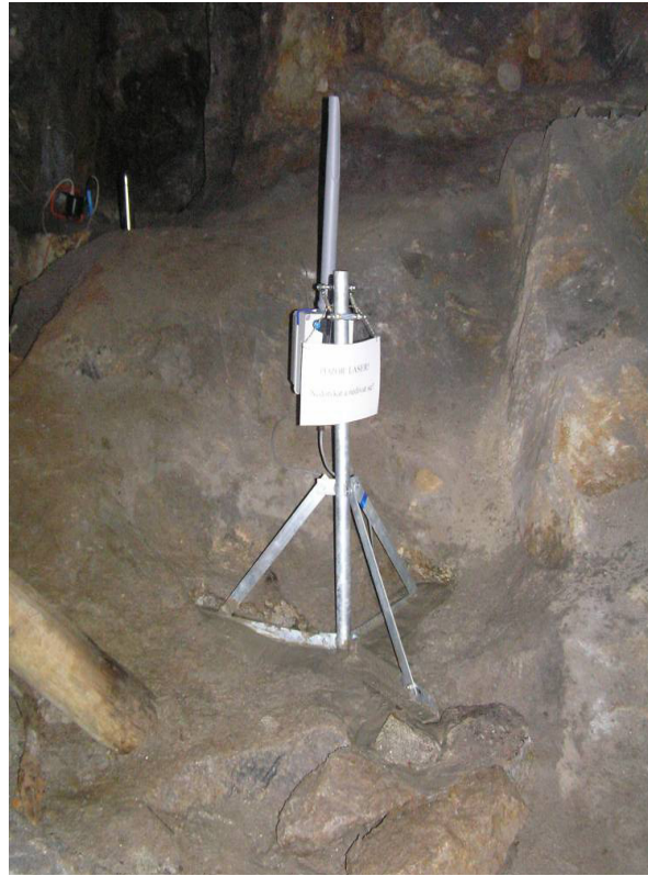
Fig. 2 LDM Leica DISTO™ A4 installed in K2 chamber.
