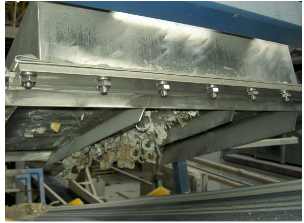
Fig. 4 The tramp iron captured by the DMON 43/48 separator.
