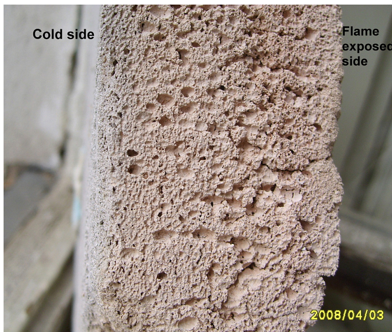
Fig. 3 Cross section of foamed FBA/smectite after thermal resistance test.
