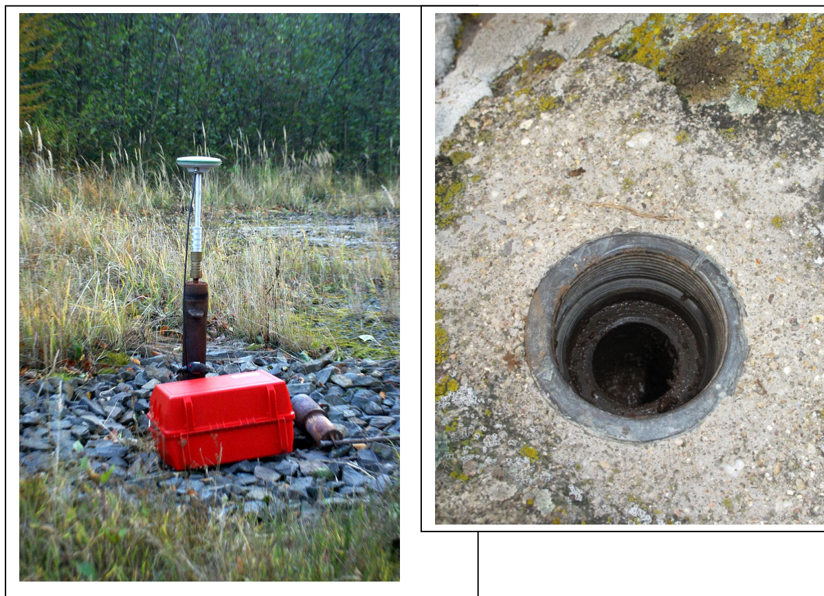
Fig. 2 Examples of point monumentations in the Morava network (Left - VRSA point, right – NAHO point).
