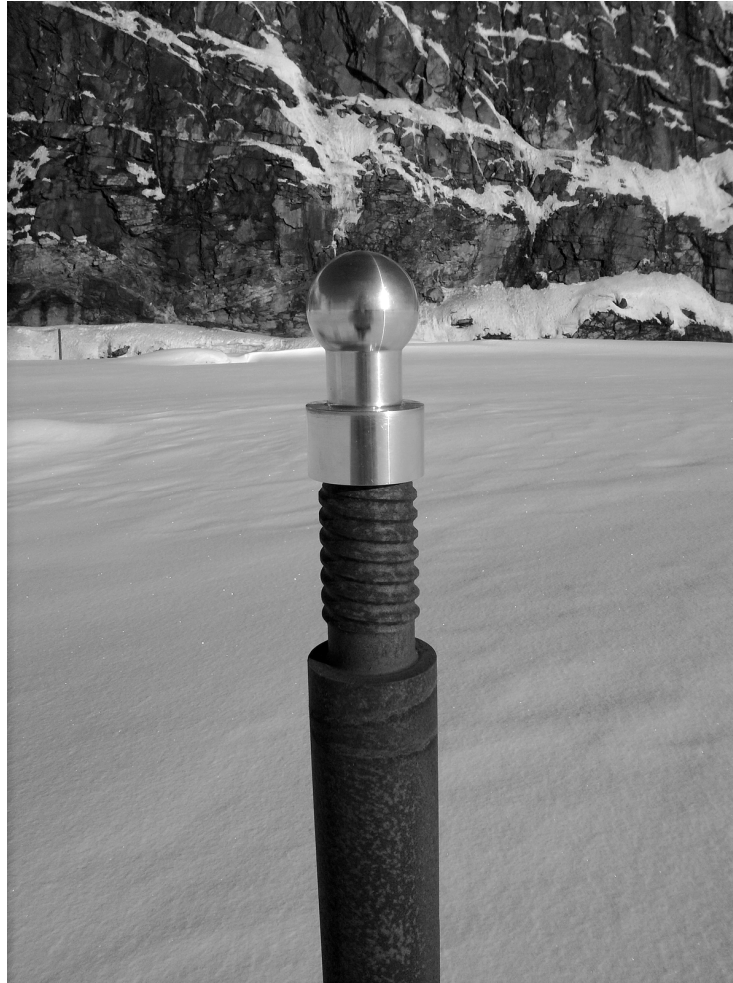
Fig. 6 Prototype of the metal sphere mounted on a drilling rod (photo Gunnar Nilsen, 2010).
