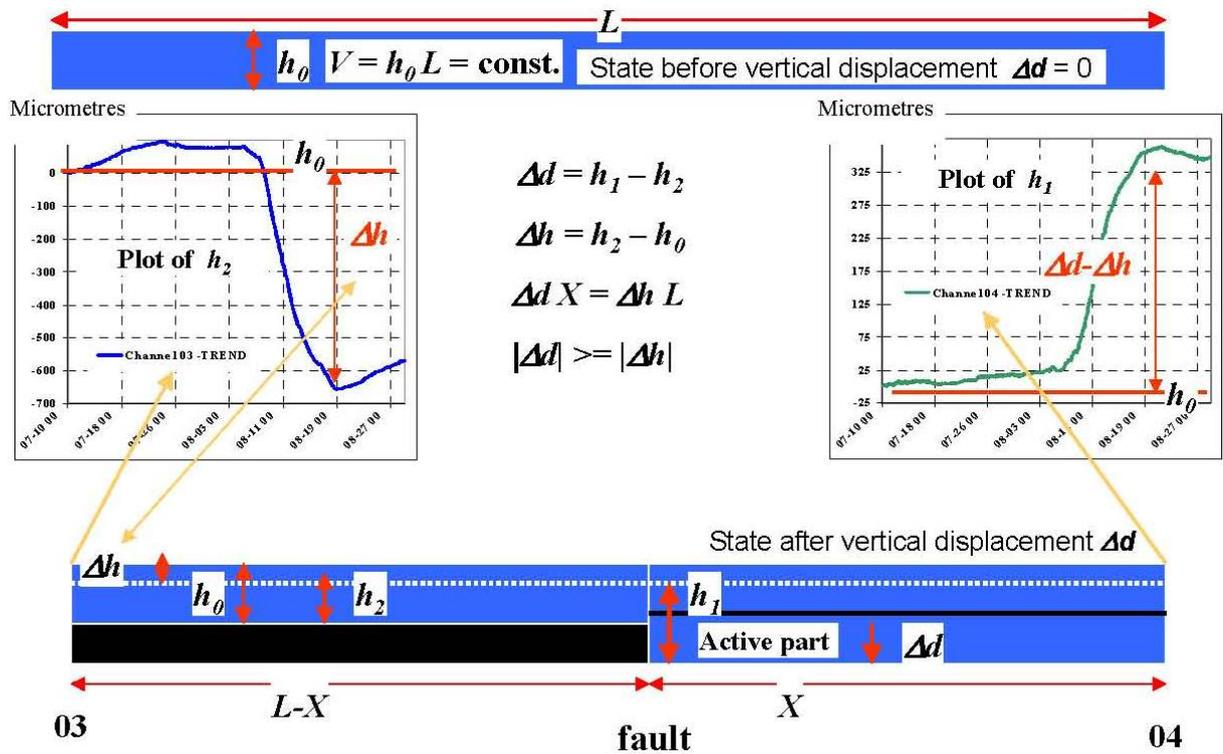
Fig. 7 A single-fault model of relative vertical displacement applied to the record of water-level changes in tiltmeter tube 03–04 during the 5<sup>th</sup> event (July 2006).
