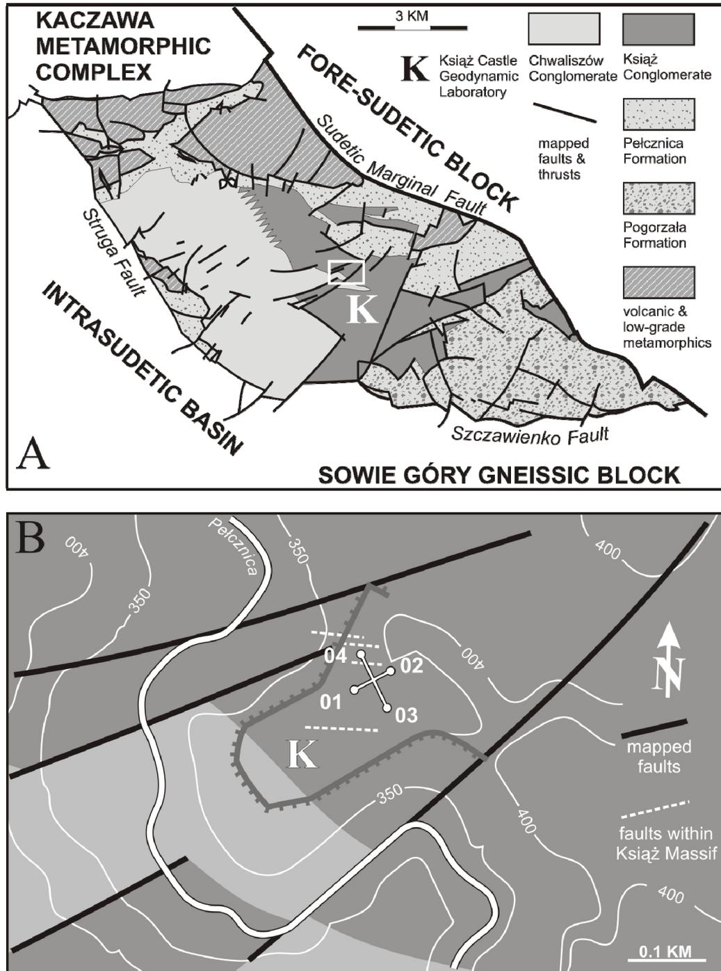
**Fig. 1** Geological map of the Świebodzice geo-structural unit with the location of the Książ Massif where the tiltmeter instrument is embedded. (B) A geological and topographic map of the Książ Massif showing the location and spatial orientation of the tiltmeter tubes 01–02 and 03–04.
