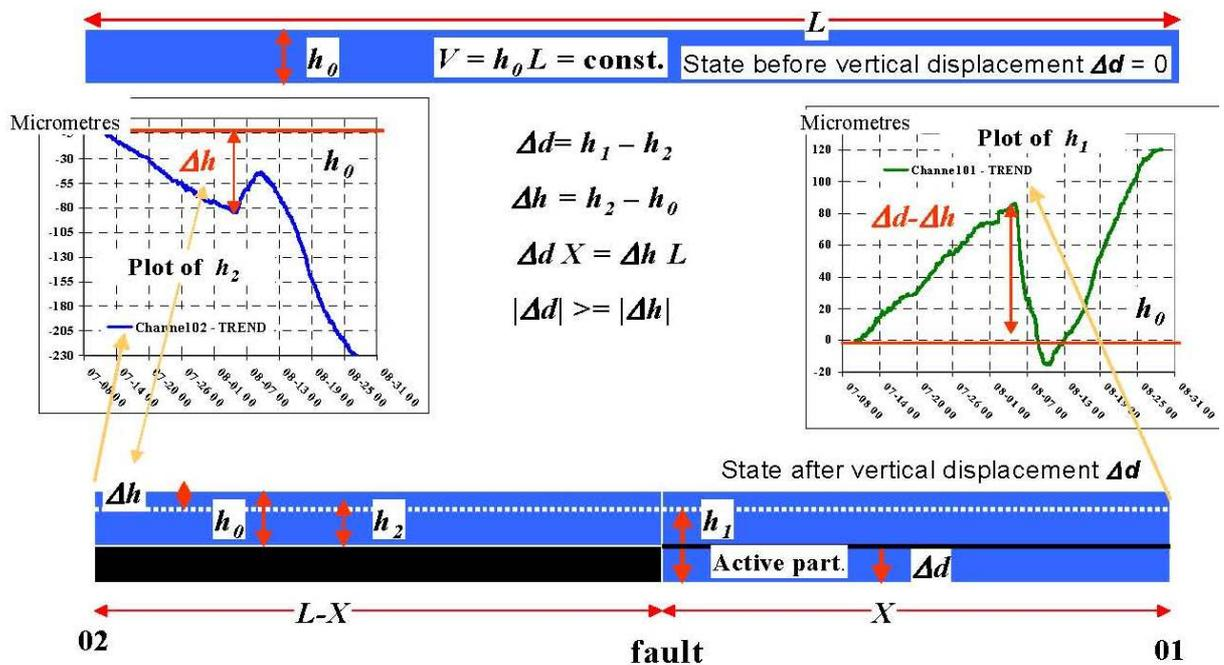
Fig. 8 A single-fault model of relative vertical displacement applied to the record of water-level changes in tiltmeter tube 01–02 during the 5<sup>th</sup> event (July 2006).
