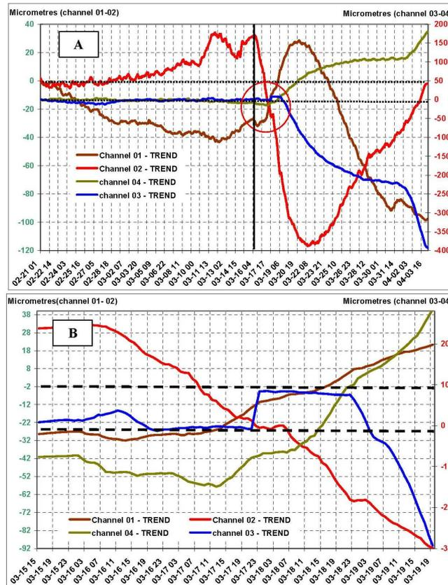
**Fig. 5** The record of strong water-level changes in tiltmeter tubes 01–02 and 03–04 (the 4<sup>th</sup> event, March 2006) after removal of tidal and evaporation signals. (B) Record from tubes 01–02 and 03–04, showing the beginning of strong signal in channels 03 and 04 and the coeval record from channels 01 and 02.
