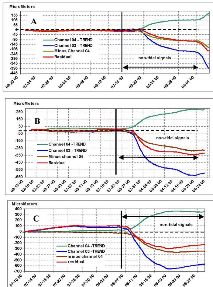
**Fig. 3** The record of strong water-level changes in tiltmeter tube 03–04 after removal of tidal and evaporation signals: (A) the 2<sup>nd</sup> event, March 2005; the 4<sup>th</sup> event, March 2006; and (C) the 5<sup>th</sup> event, July 2006.
