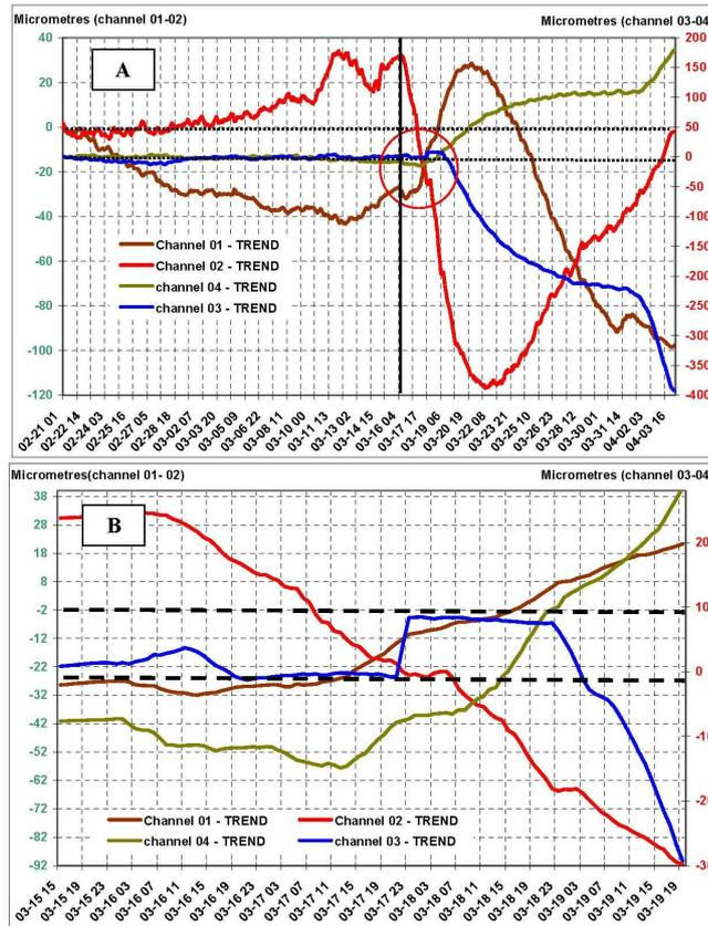
**Fig. 4** The record of strong water-level changes in tiltmeter tubes 01–02 and 03–04 (the 2<sup>nd</sup> event, March 2005) after removal of tidal and evaporation signals. (B) Record from tubes 01–02 and 03–04, showing the beginning of strong signal in channels 03 and 04 and the coeval record from channels 01 and 02.
