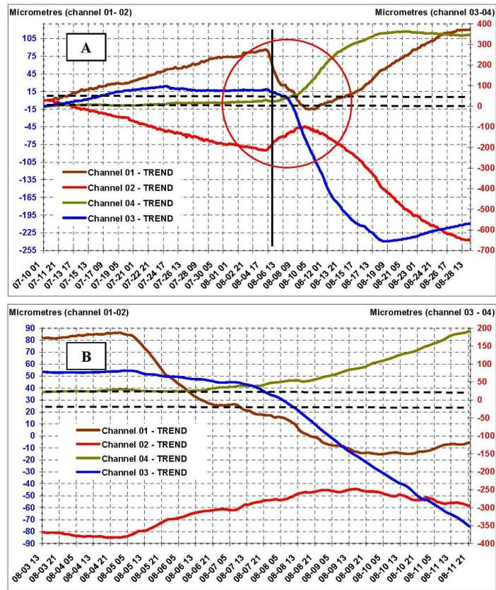
**Fig. 6** The record of strong water-level changes in tiltmeter tubes 01–02 and 03–04 (the 5<sup>th</sup> event, July 2006) after removal of tidal and evaporation signals. (B) Record from tubes 01–02 and 03–04, showing the beginning of strong signal in channels 03 and 04 and the coeval record from channels 01 and 02.
