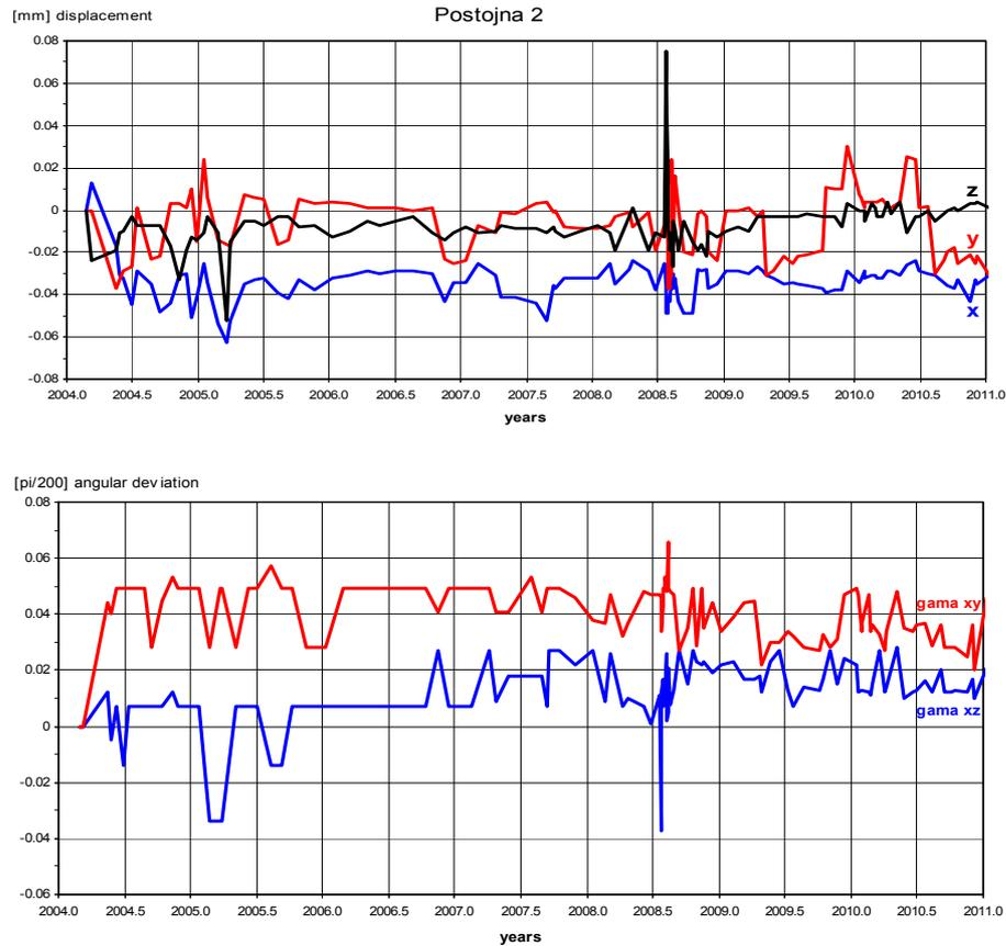
**Fig. 7** Relative displacements (+ $x$  compression (- $x$  extension), + $y$  sinistral horizontal movement (- $y$  dextral) and + $z$  down-slip of NE block (- $z$  uplift) and angular deviation detected with a TM 71 extensometer for Postojna 2 (Postojna cave).
