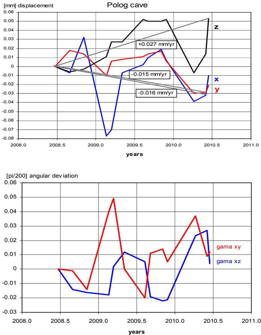
**Fig. 8** Relative displacements (+ $x$  compression (- $x$  extension), + $y$  sinistral horizontal movement (- $y$  dextral) and + $z$  uplift of NW block (- $z$  down-slip)) and angular deviation detected with a TM 71 extensometer for Polog cave.
