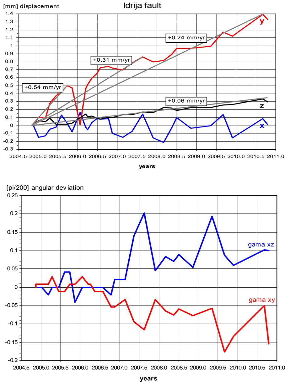
**Fig. 2** Relative displacements (+x compression (-x extension), +y sinistral horizontal movement (-y dextral) and +z down-slip of SW block (-z uplift)) and angular deviation detected with a TM 71 extensometer for the Idrija fault (Učja).
