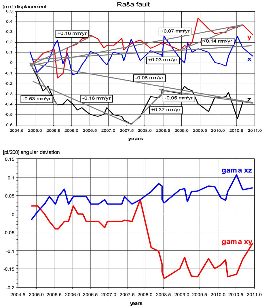
**Fig. 4** Relative displacements (+ $x$  compression ( $-x$  extension), + $y$  sinistral horizontal movement ( $-y$  dextral) and + $z$  down-slip of SW block ( $-z$  uplift)) and angular deviation detected with a TM 71 extensometer for the Raša fault (Vremščica).
