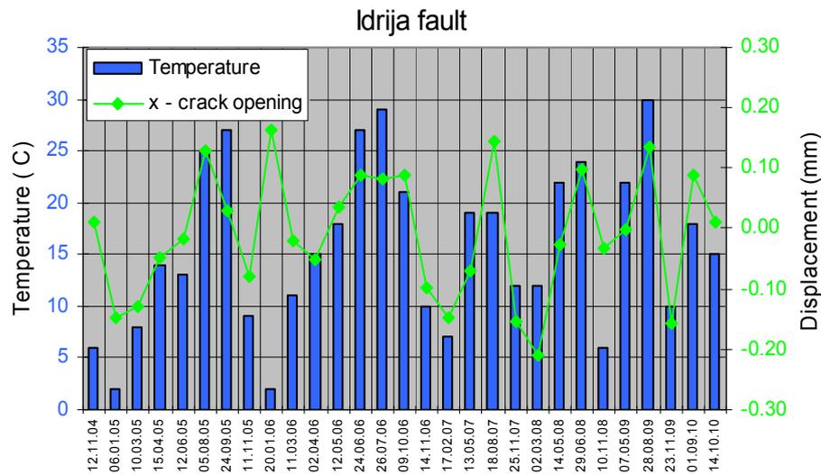
**Fig. 3** Correlation between temperature variations and opening ( $-x$  extension) and closing ( $+x$  compression) of the crack at the Idrija fault (Učja) monitoring site.
