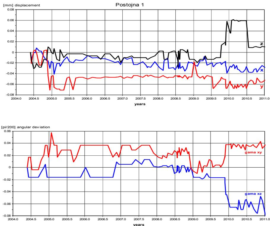
**Fig. 6** Relative displacements (+ $x$  compression (- $x$  extension), + $y$  sinistral horizontal movement (- $y$  dextral) and + $z$  down-slip of NE block (- $z$  uplift) and angular deviation detected with a TM 71 extensometer for Postojna 1 (Postojna cave).
