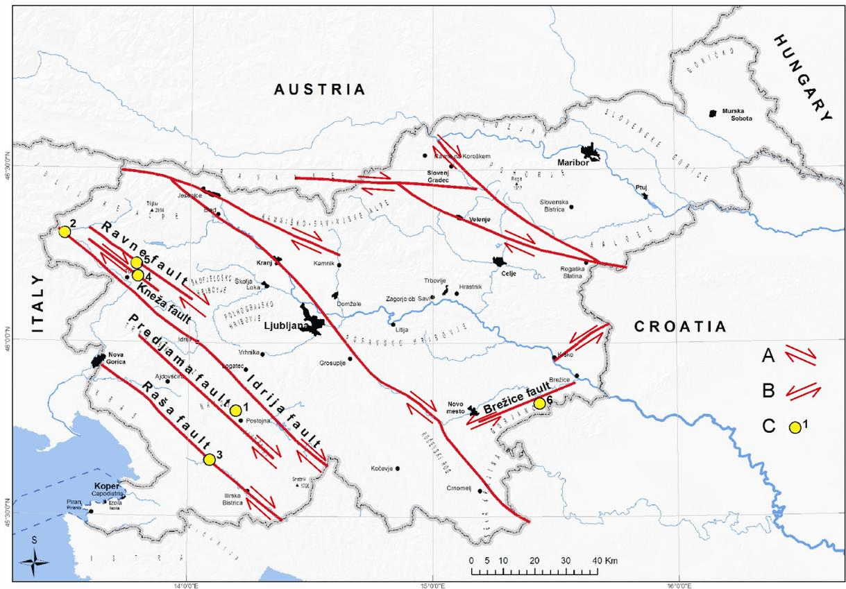
**Fig. 1** TM 71 monitoring sites in Slovenia and most important faults. A – dextral horizontal movement along the fault, B – sinistral horizontal movement along the fault, C – monitoring sites (1-Postojna cave, 2-Učja, 3-Vremščiča, 4-Zadlazi-Čadrg, 5-Polog cave, 6-Kostanjevica cave).
