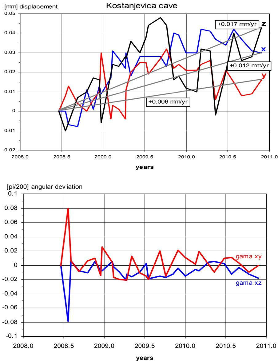
**Fig. 9** Relative displacements (+x compression (-x extension), +y sinistral horizontal movement (-y dextral) and +z down-slip of NW block (-z uplift)) and angular deviation detected with a TM 71 extensometer for Kostanjevica cave.
