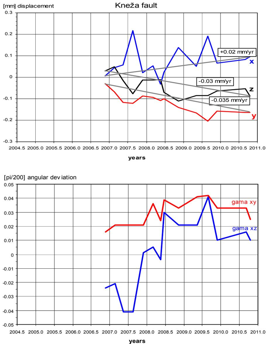
**Fig. 5** Relative displacements (+x compression (-x extension), +y sinistral horizontal movement (-y dextral) and +z down-slip of SW block (-z uplift)) and angular deviation detected with a TM 71 extensometer for the Kneža fault (Zadláz-Čadrg).
