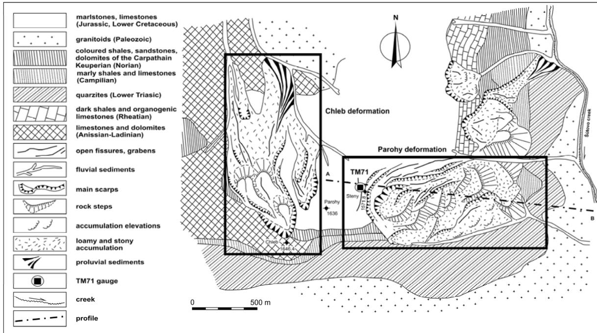
**Fig. 1** Geological map showing the location of the TM71 and the area surrounding the Parohy Site (after Nemčok, 1973).
