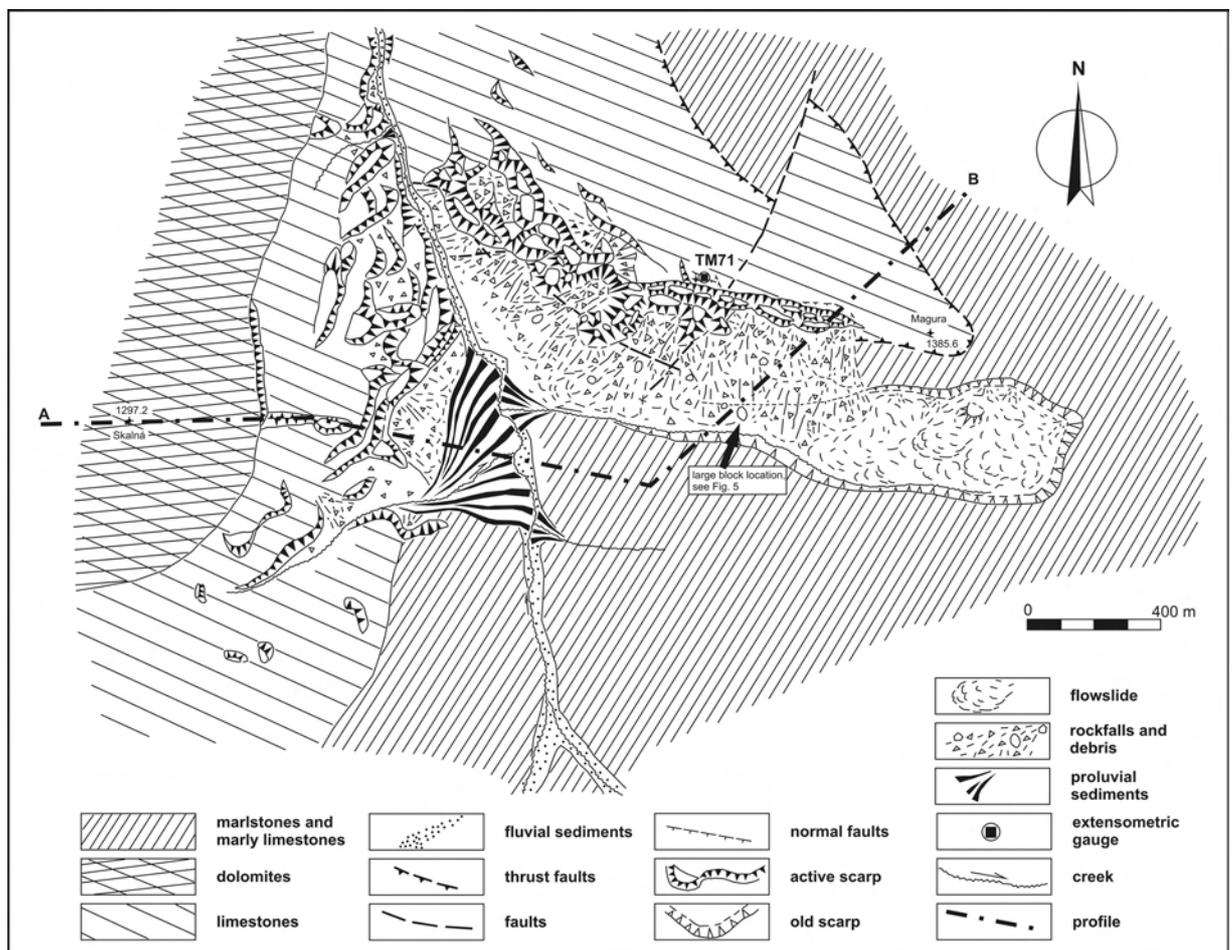
**Fig. 6** Geological map showing the location of the TM71 and the area surrounding the Štrochy Site (modified after Nemčok, 1982).
