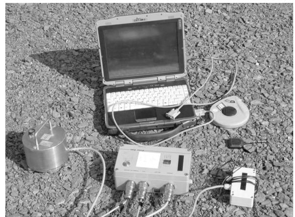
Fig. 6 Seismic station GAIA by VISTEC Praha with ViGeo2 sensor
