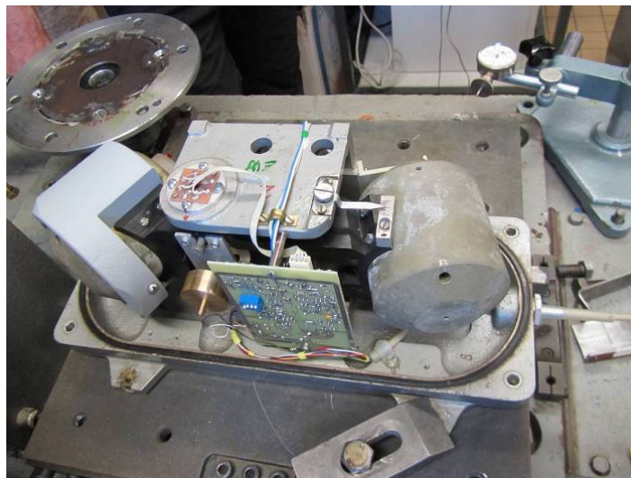
Fig. 4 The S-5-SR seismometer anchored on the translation movement desk during laboratory tests; links - rotational desk.
