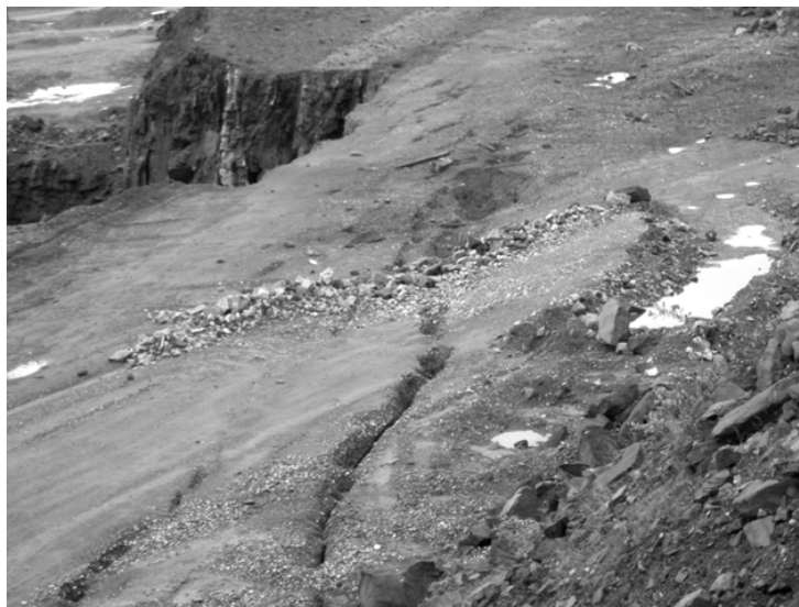
Fig. 9 Fractures on the hanging wall in the A line area (caved in part of the hanging wall in the background).
