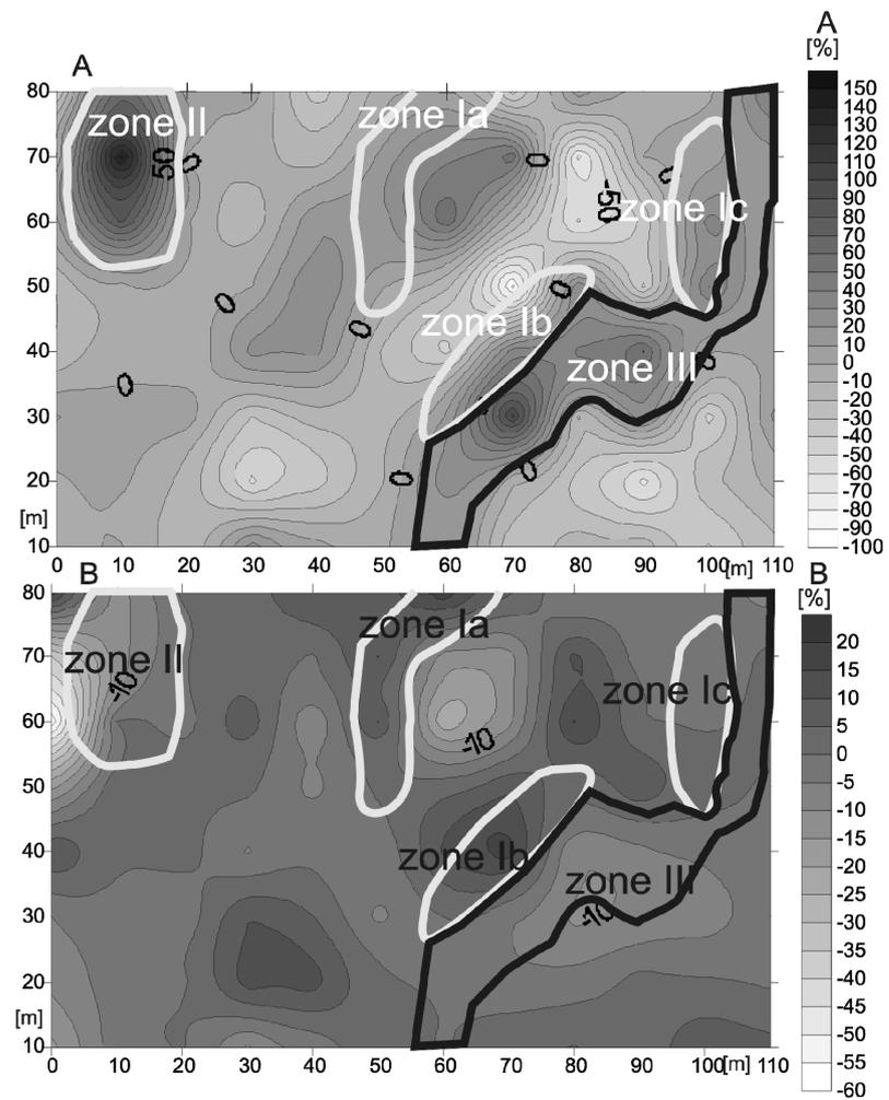
**Fig. 5** Map of electromagnetic measurements – area 3, A - in-phase data, B - quadrature data, zone Ia, Ib, Ic, II - contaminated water, zone III – uncontaminated zone.
