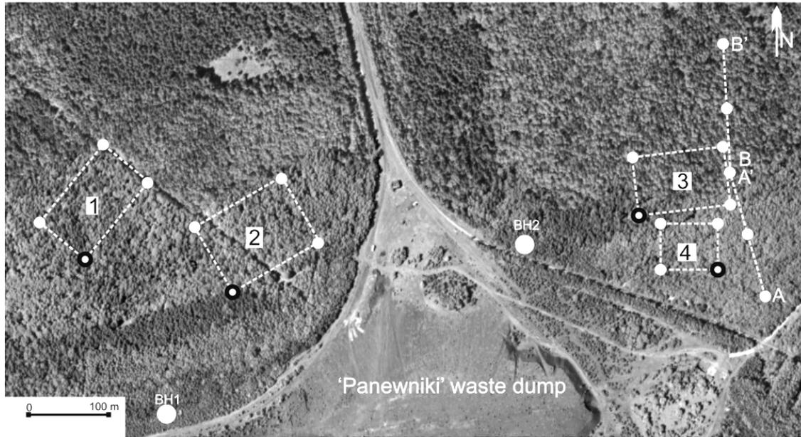
**Fig. 2** Area of investigation in Southern Poland - "Panewniki" waste dump, A-A', B-B' – geoelectrical profiles, 1-4 area of electromagnetic measurements, BH1 and BH2 – lithological profiles.
