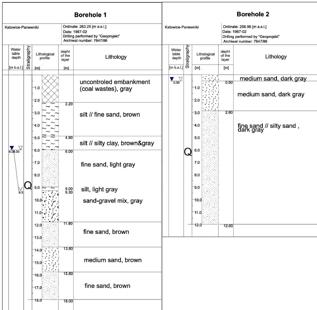
**Fig. 1** Archival lithological profiles (borehole 1 - BH1 and borehole 2 - BH2) carried out by “Geoprojekt Katowice” company.
