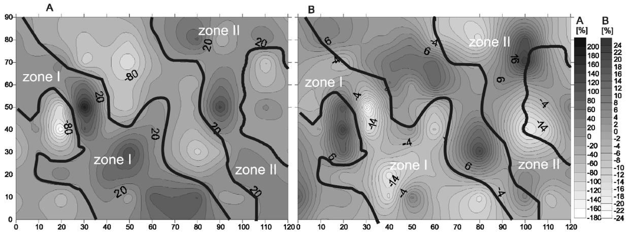
**Fig. 4** Map of electromagnetic measurements – area 2, A - in-phase data, B - quadrature data zone I-II – uncontaminated zone.
