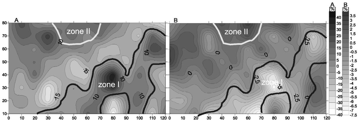
**Fig. 3** Map of electromagnetic measurements – area 1, A - in-phase data, B - quadrature data, zone I – uncontaminated zone, zone II – contaminated water.
