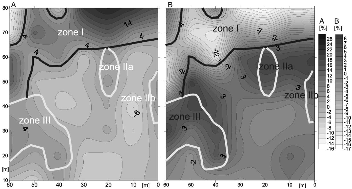
**Fig. 6** Map of electromagnetic measurements – area 4, A - in-phase data, B - quadrature data, zone I – water uncontaminated, zone IIa, IIb, III – contaminated water.
