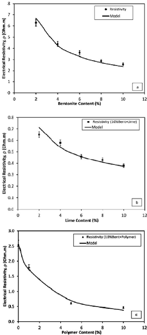
**Fig. 7** Variation of electrical resistivity with bentonite and modifier contents (a) untreated ultra-soft soil, (b) 10 % bentonite ultra-soft soil treated with lime and (c) 10 % bentonite ultra-soft soil treated with polymer(bars represent the standard deviation).
