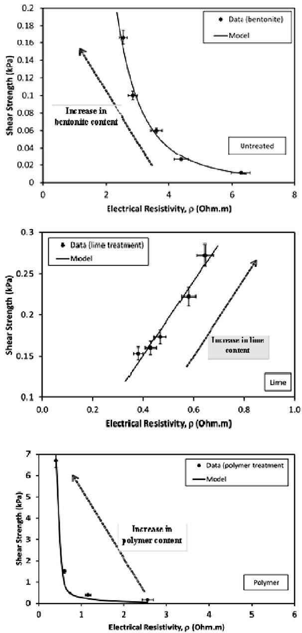
**Fig. 8** Variation of the shear strength with electrical resistivity (a) untreated ultra-soft soil, (b) treated 10% bentonite ultra-soft soil with lime and (c) treated 10% bentonite ultra-soft soil with polymer(bars represent the standard deviation).
