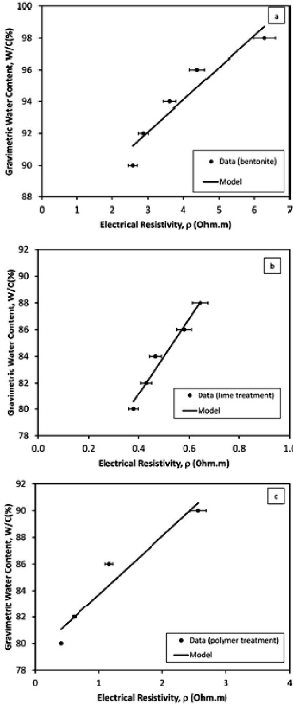
**Fig. 9** Variation of gravimetric water content with electrical resistivity (a) untreated ultra-soft soil, (b) 10% bentonite ultra-soft soil treated with lime and (c) 10% bentonite ultra-soft soil treated with polymer (bars represent the standard deviation).
