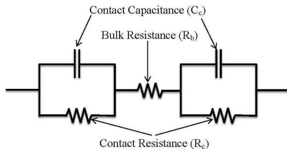
**Fig. 1** The correspondance electrical circuit simulating the ultra-soft soil condition.
