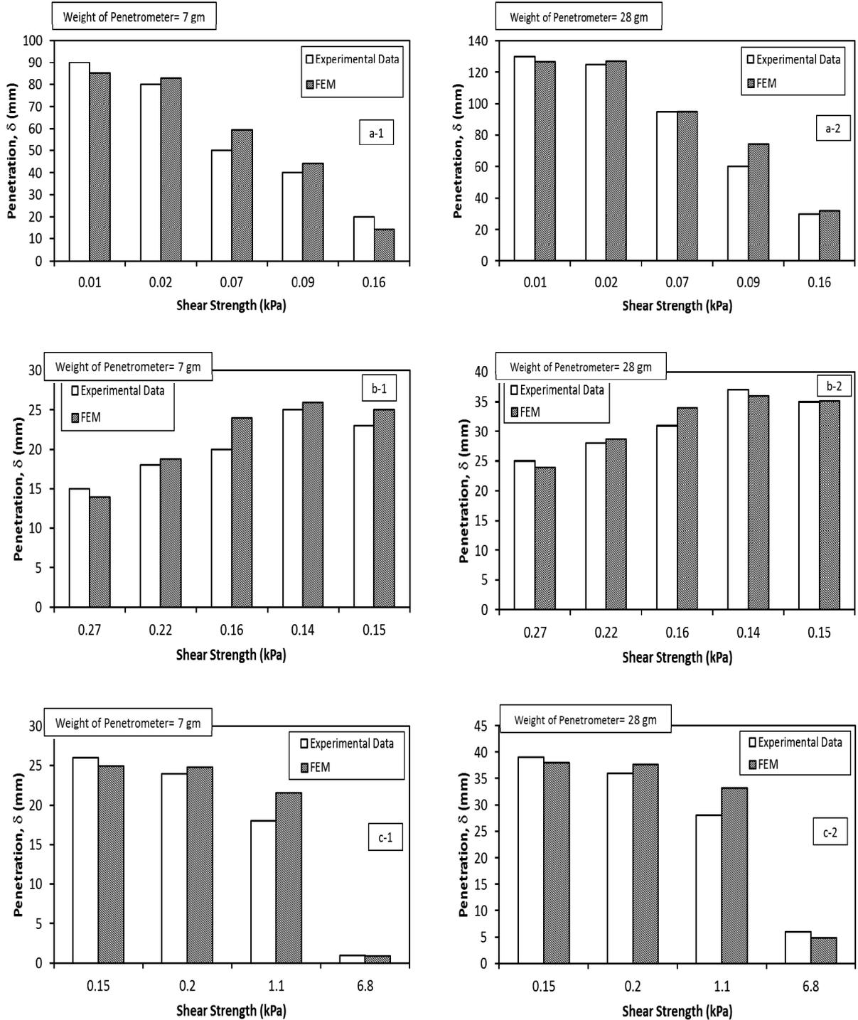
**Fig. 10** Comparing the predicted (FEM) and experimental CIGMAT miniature penetrometer penetration (a) untreated ultra-soft soil (b) 10 % bentonite ultra-soft soil treated with lime, and (c) 10 % bentonite ultra-soft soil treated with polymer.
