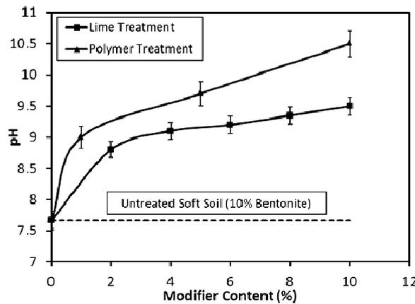
**Fig. 6** Variation of pH with modifier content (lime and polymer) for 10 % bentonite ultra-soft soil (bars represent the standard deviation).**(iii) Polymer treatment**
