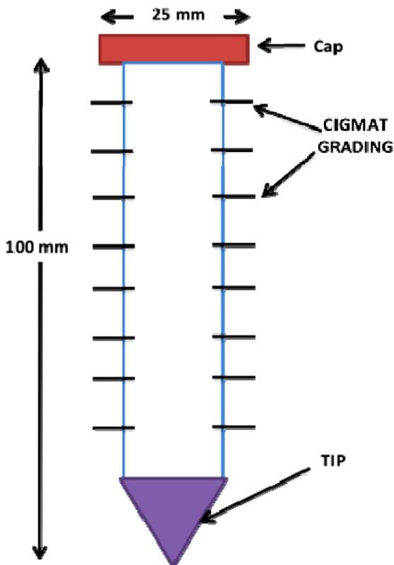
**Fig. 3** Schematic of the miniature CIGMAT penetrometer.
