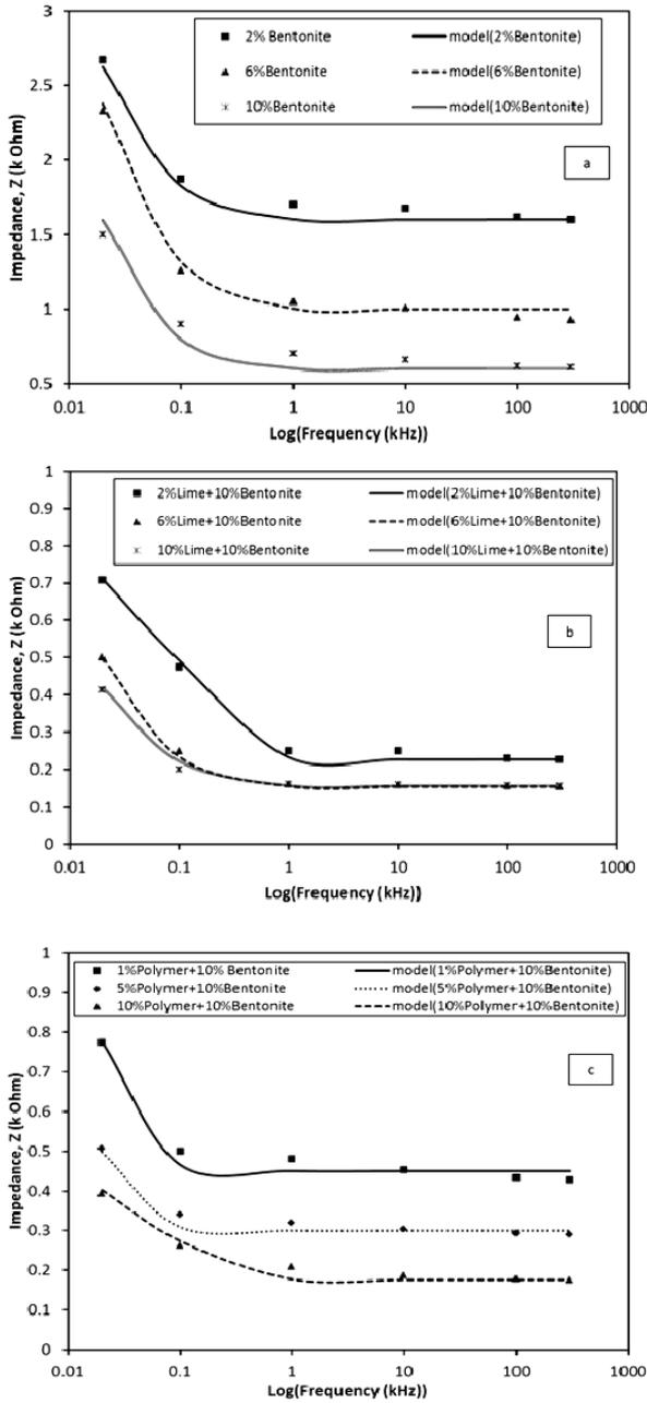
**Fig. 2** Predicted and measured impedance frequency relationship (a) untreated ultra-soft soil, (b) 10 % bentonite ultra-soft soil treated with lime and (c) 10 % bentonite ultra-soft soil treated with polymer (Raheem et al., 2017).
