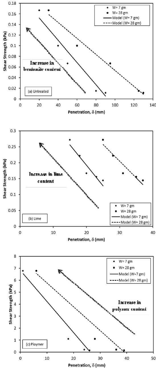
**Fig. 5** Relationship between shear strength and CIGMAT penetrometer penetration (a) untreated ultra-soft soil, (b) 10 % bentonite ultra-soft soil treated with lime and (c) 10 % bentonite ultra-soft soil treated with polymer.
