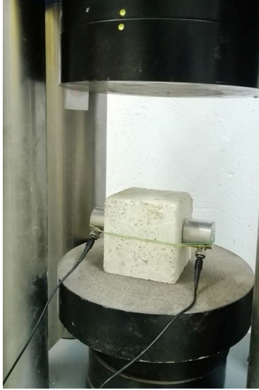
Fig. 3 Uniaxial compression apparatus with ultrasonic transducers.
