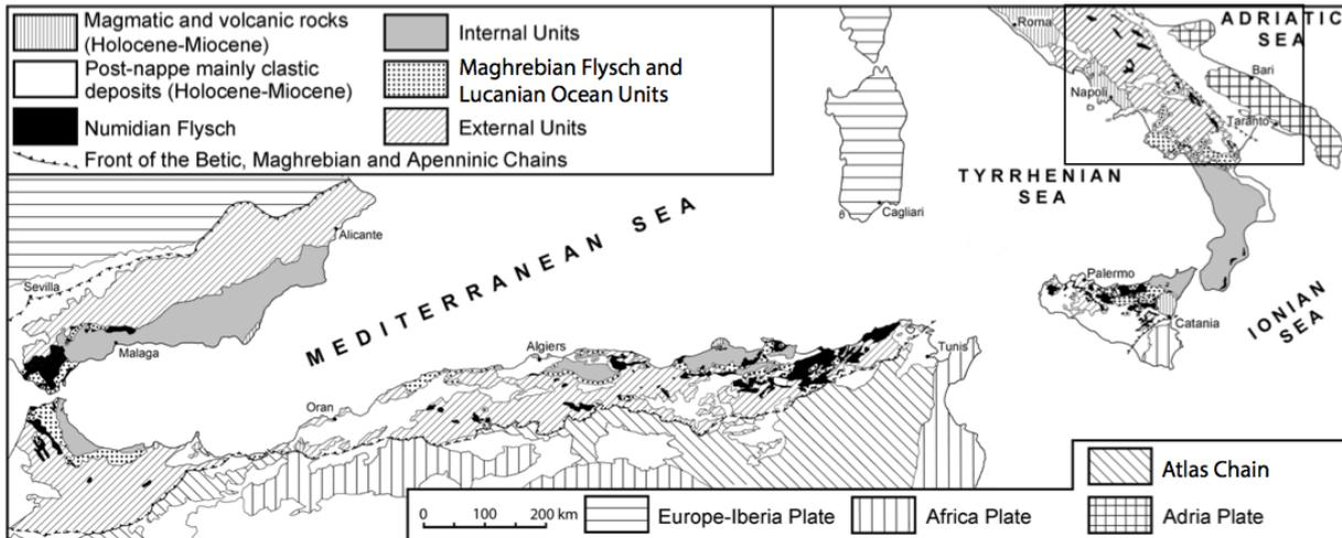
**Fig. 1** Schematic geological map of Numidian Flysch outcropping in Western-Central Mediterranean area (modified from Hoyez (1989)). The box on the right indicates the studied area showed in Figure 2.
