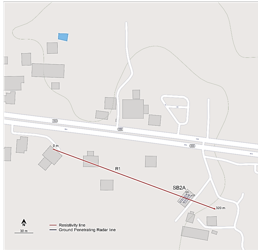
Fig. 3 2-D resistivity and GPR survey lines in the study area of SB2A.
