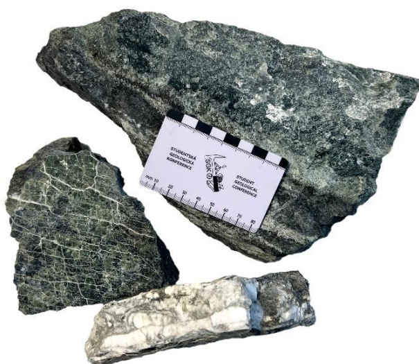
Fig. 1 Specimens of serpentinite S1 taken from the site, together with a piece of magnesite vein. Scale for comparison (black & white rectangles equals 1 cm).
