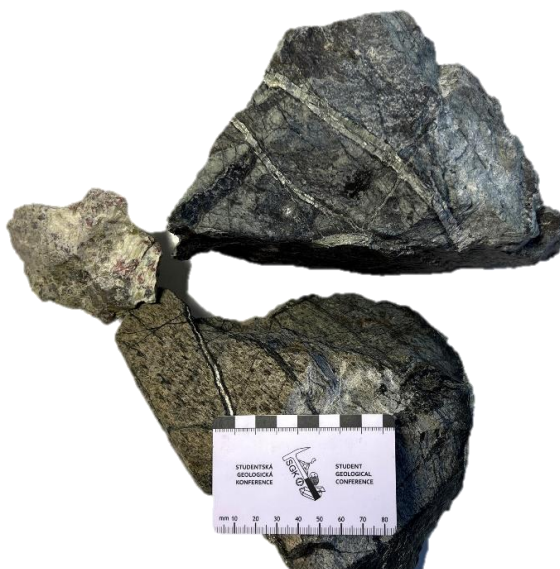
Fig. 2 Specimens of serpentinite S2 taken from the site, with intersecting light-coloured chrysotile veins. Scale for comparison (black & white rectangles equals 1 cm).
