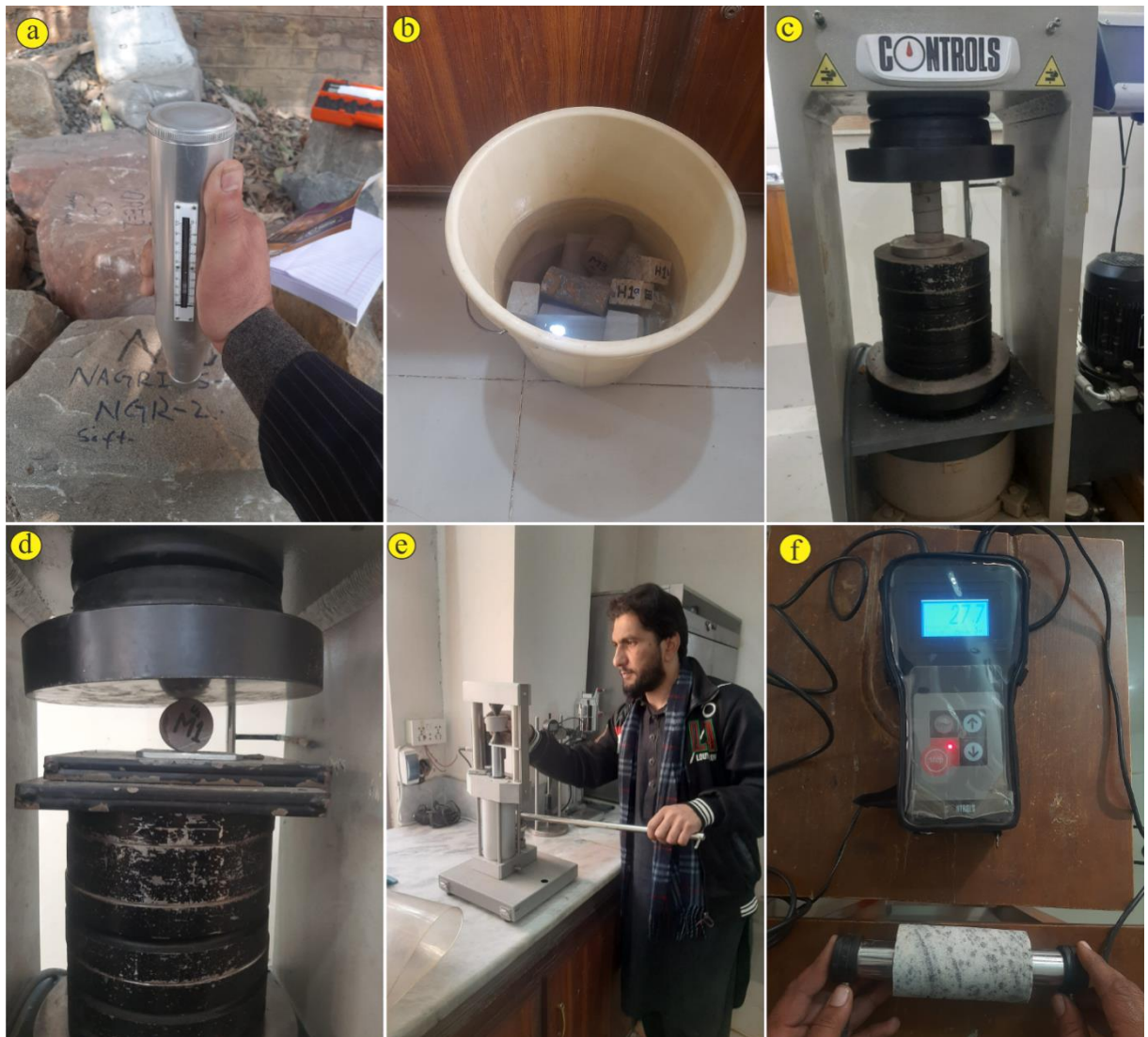
Fig. 3 Photographs showing various geotechnical tests. a) showing Schmidt hammer test of the bulk samples; b) showing Water absorption test of the core samples; c) showing Unconfined Compressive Strength test of the core samples; d) showing Unconfined Tensile Strength test of the core samples; e) showing Point Load Test of the core samples; f) showing Ultrasonic Pulse Velocity test of the core samples.
