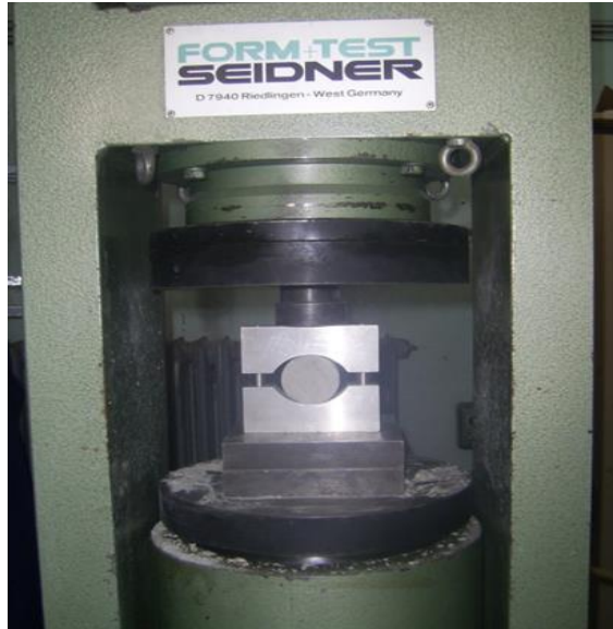
Fig. 6 Hydraulic press used for the strength test.
