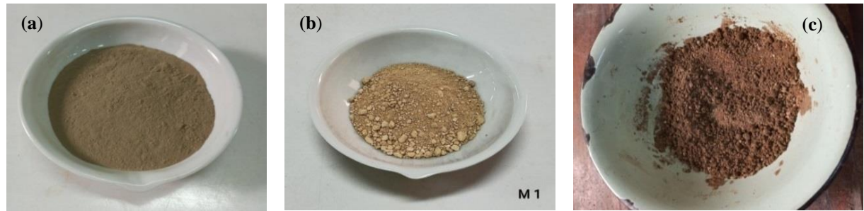
Fig. 7 Materials used for mixtures preparation: (a) Silty fines; (b) Dry Tuff sample; (c) Moisturized Tuff/fines mixtures.
