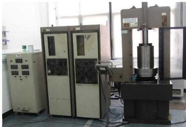
Fig. 2 The 815.02 rock mechanics testing system.
