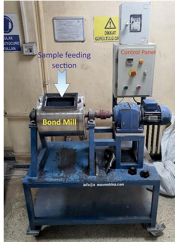
Fig. 10 Laboratory Bond mill used in this study.
