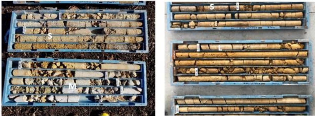
Fig. 3 General view of the cores obtained from core drilling in the study area.
