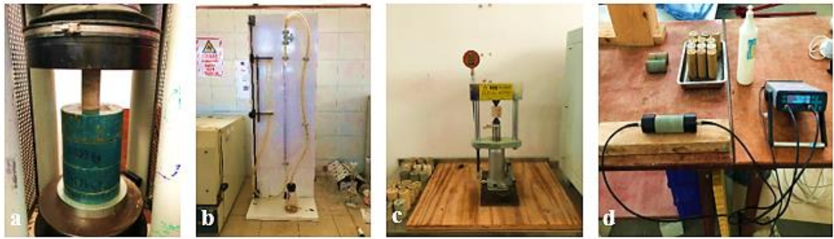
Fig. 4 a) uniaxial compressive strength test, b) Bernard calcimeter, c) point load strength test, d) pundit lab ultrasonic pulse velocity test.
