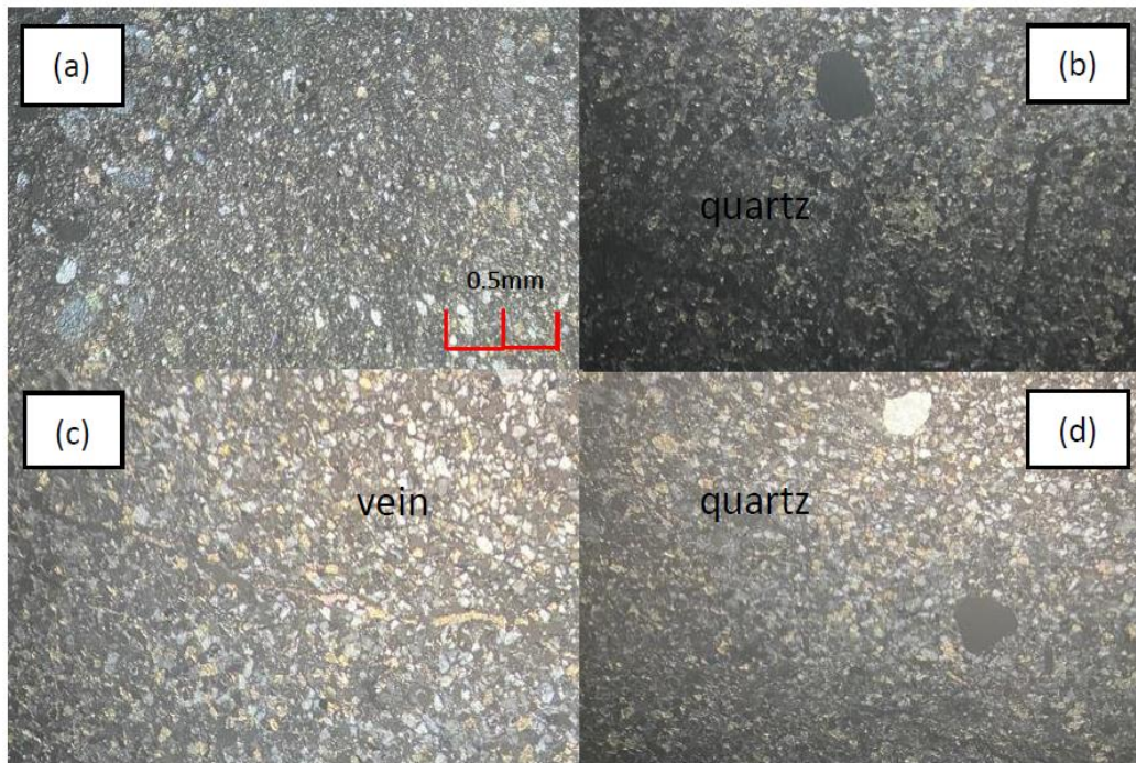
Fig. 15 Thin section photomicrographs of sandstone 1 rock which consists of vein and quartz minerals.
