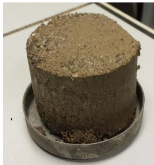
Fig. 11 Sample of Carbonate sand after an oedometric test at 30 MPa.
