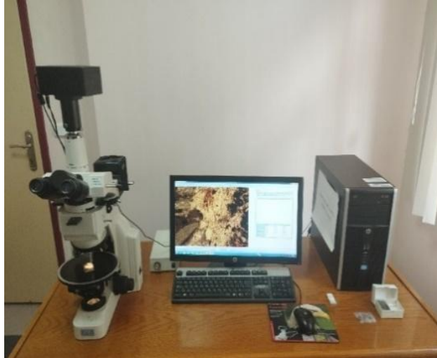
Fig. 1 Polarizing microscope used for photographing and examining thin sections of samples.
