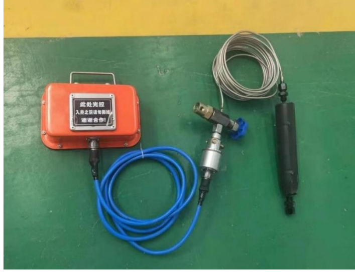
Fig. 2 YHY-60 Infrared Memory-Type Borehole Stress Meter Used for Data Acquisition.
