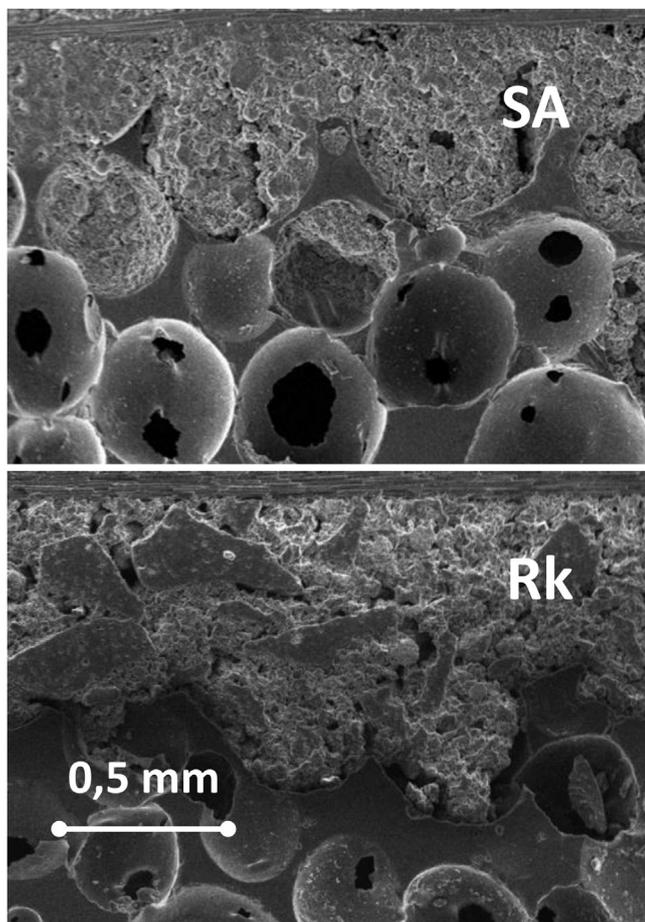
**Fig. 2.** The fine grain size of the unprocessed SA adhesive allows the formation of a thinner bonding layer and better filling of the pores; above SA adhesive, below Rk adhesive – both structures after high-temperature curing at 1000 °C (SEM micrograph).
