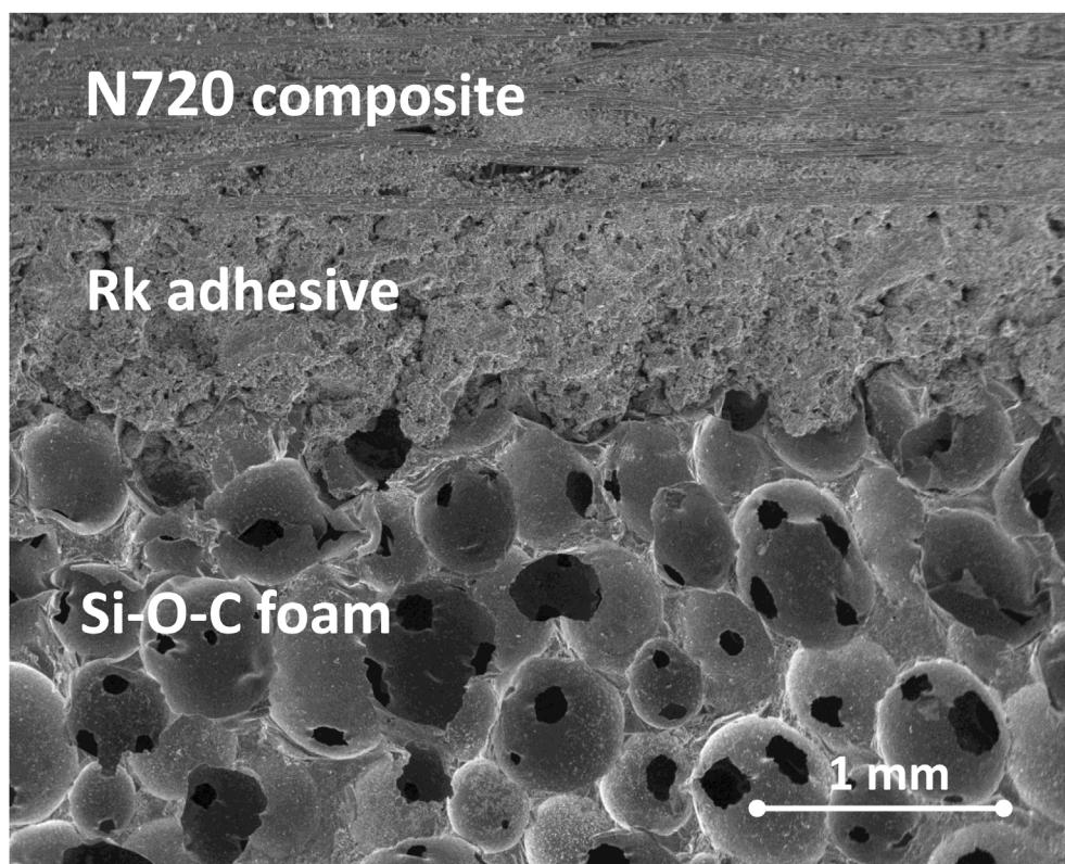
**Fig. 1.** Adhesive connection between the Si–O–C foam core and the CMC composite skin after high temperature curing at 1000 °C (SEM micrograph).
