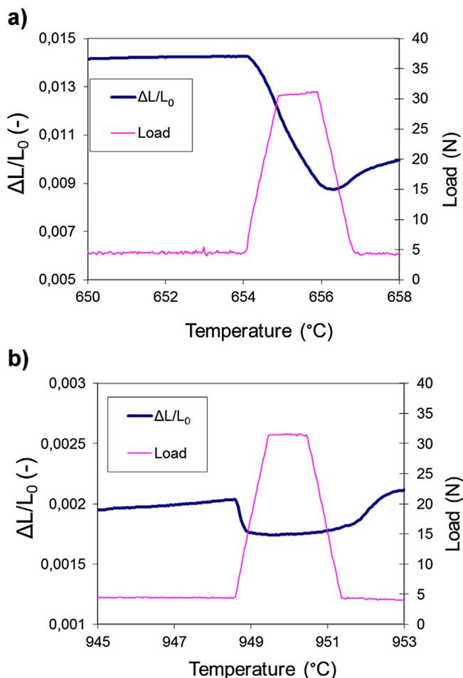
Fig. 7. Detail of one load cycle from Fig. 6: a) cycle at 650 °C; b) cycle at 950 °C.
