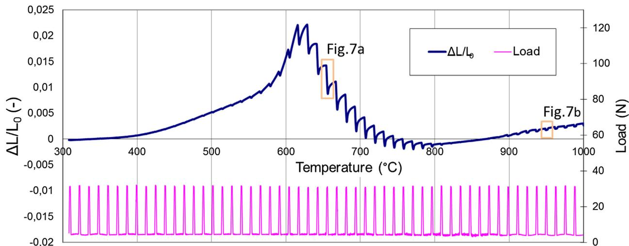
Fig. 6. Experiment studying the rheological and dimensional changes during the high-temperature cure of the alumino-silicate adhesive (material: SA adhesive), by applying cyclic load.
