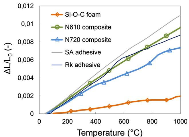
**Fig. 5.** Thermal dilations of alternatively used sandwich components in their thermally stabilised state (post-cure, post pyrolysis).
