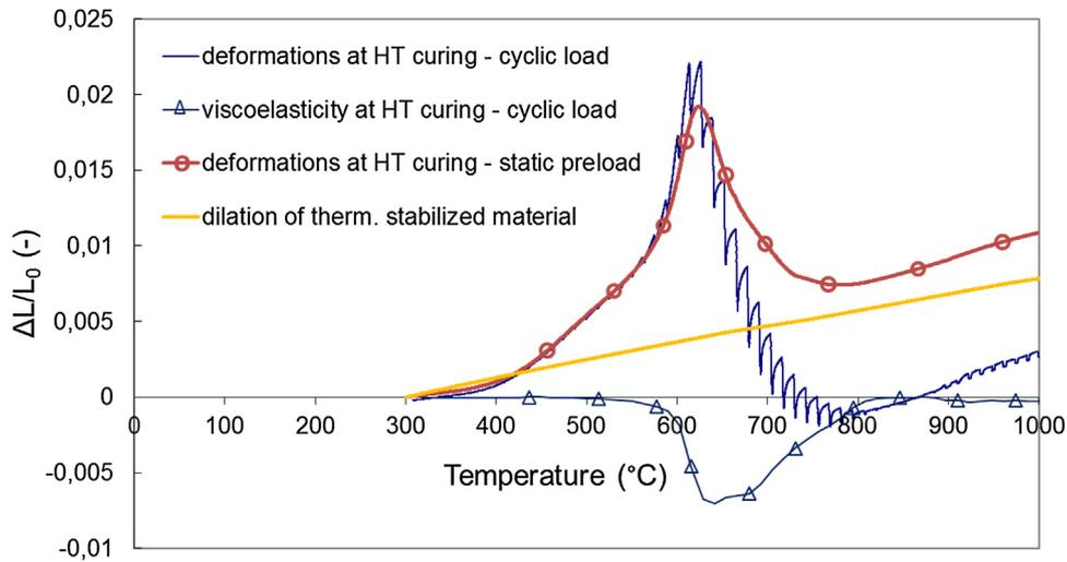
Fig. 8. Rheological behaviour and thermally induced dilations of the SA adhesive.
