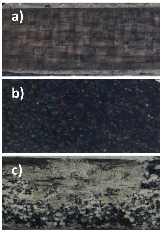
**Fig. 10.** Examples of fracture types in the prepared sandwiches, differing in fracture location: a) in composite b) in the foam and c) in adhesive.
