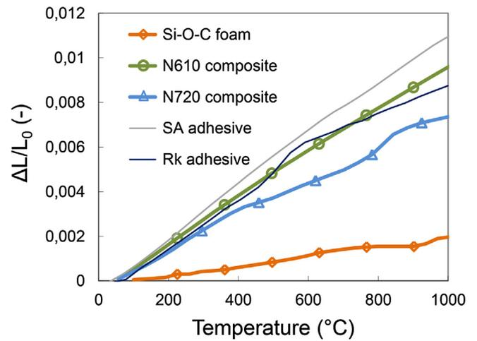
Fig. 5. Thermal dilations of alternatively used sandwich components in their thermally stabilised state (post-cure, post pyrolysis).
