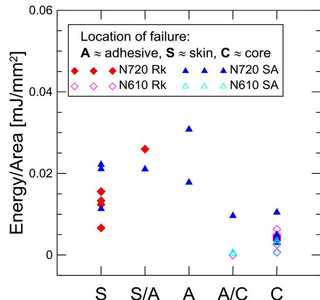
**Fig. 11.** Results of the DCB test, i.e., normalised work of fracture sorted by fracture location.
