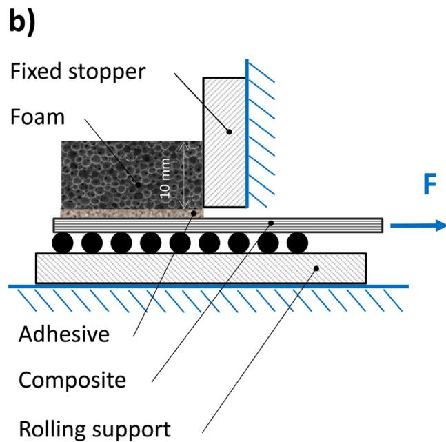
Fig. 4. Experimental setup for mechanical tests of adhesive bond between skin and core: a) modified DCB test and b) shear test.
