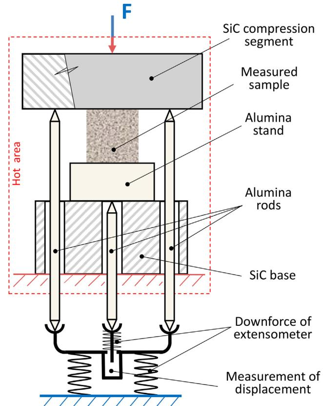
**Fig. 3.** Experimental setup for the characterization of the rheological behaviour and of the thermally induced dimensional changes of the studied adhesives.
