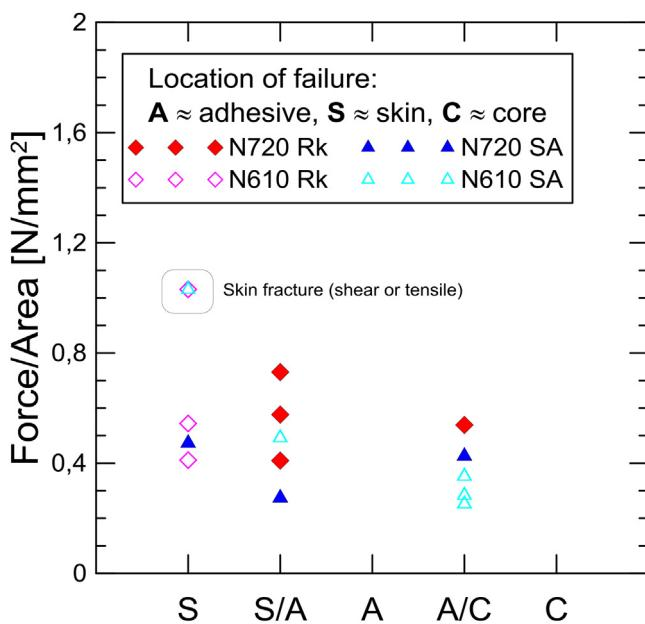
**Fig. 12.** Normalized decohesion force obtained from the shear test, sorted by fracture location.
