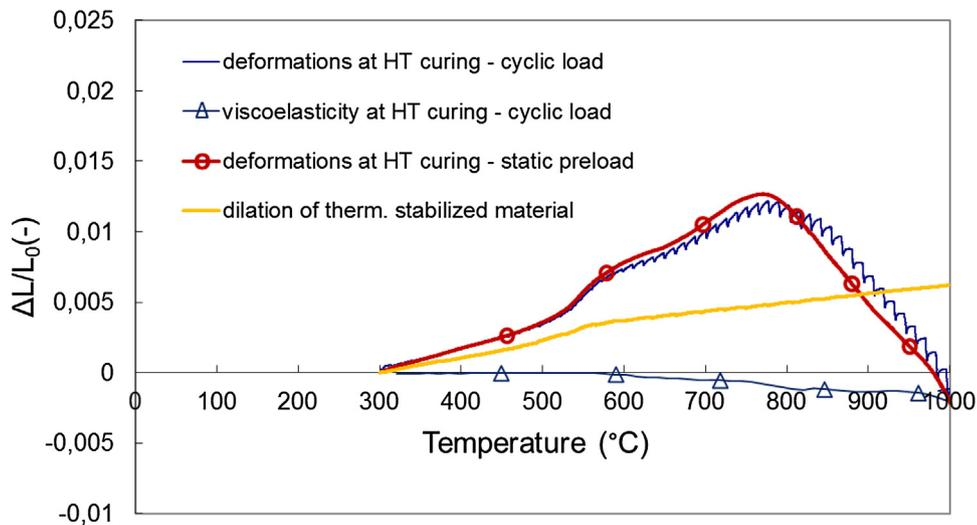
Fig. 9. Rheological behaviour and thermally induced dilations of the Rk adhesive.
