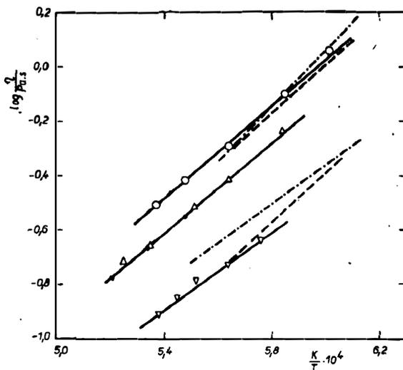
Fig. 2. Viscosity of the melts of  $\text{CaSiO}_3$ ,  $\text{CaMgSi}_2\text{O}_6$  and  $\text{Ca}_2\text{MgSi}_2\text{O}_7$ .  $\circ$  —  $\text{CaMgSi}_2\text{O}_6$ ,  $\Delta$  —  $\text{CaSiO}_3$ ,  $\nabla$  —  $\text{Ca}_2\text{MgSi}_2\text{O}_7$ , - - - - after [19], — after [20],  $\bullet$  — after [21], full lines according to equations (5)–(7).
