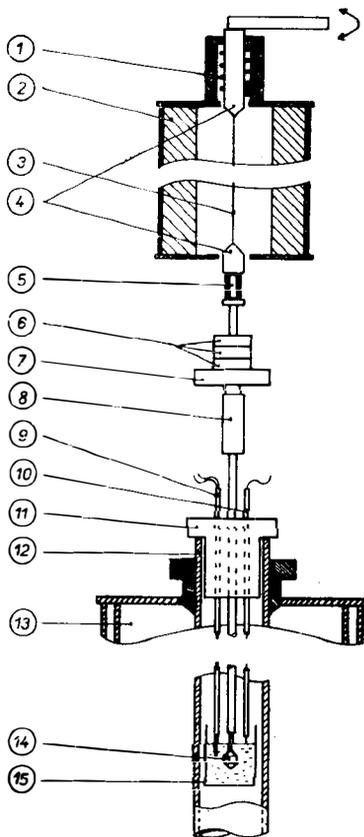
Fig. 1. Schematic sectional view of the oscillation viscometer. 1 — winding device, 2 — tempered protective jacket of the torsion wire, 3 — torsion wire, 4 — gripping collets, 5 — mirror, 6 — additional brass rings, 7 — heavy ring of stainless steel, 8 — bayonet letting down device, 9 — thermocouple, 10 — level surface contact, 11 — furnace closure, 12 — corundum furnace shaft, 13 — water-cooled furnace, 14 — measuring body, 15 — crucible with melt.
