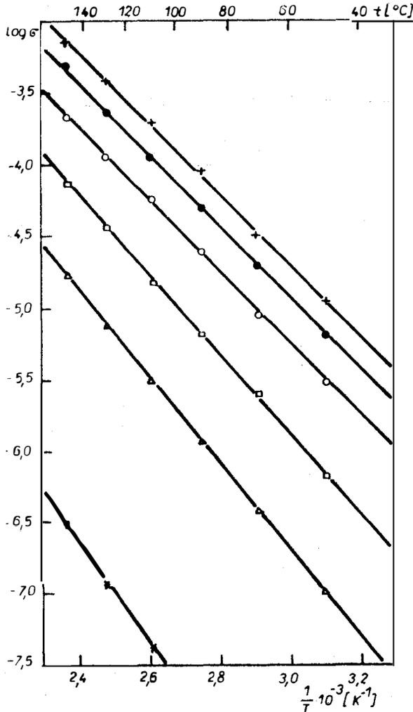
Fig. 3. Temperature dependence of electrical conductivity of glasses having the composition  $X \text{Li}_2\text{Cl}_2-3 \text{Li}_2\text{O}-7 \text{B}_2\text{O}_6$
