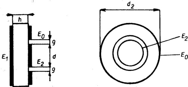
Fig. 1. Schematic diagram of the arrangement of electrodes on the specimen for measuring the electrical conductivity by the three-point method.
