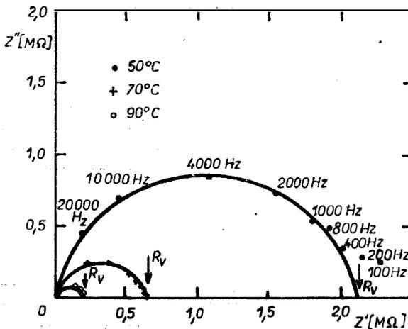
Fig. 2. Typical impedance spectrum of glasses in the system  $\text{Li}_2\text{Cl}_2\text{—Li}_2\text{O—B}_2\text{O}_3$ .
