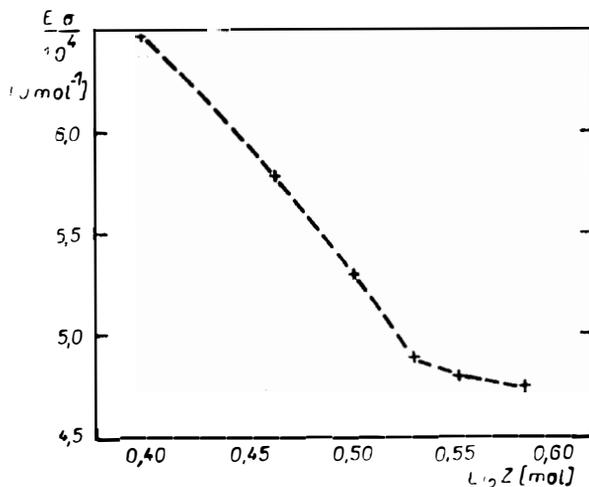
Fig. 6.  $E_a$  vs.  $\text{Li}_2\text{Z}$  content in glasses having the composition  $X \text{Li}_2\text{Cl}_2 - 3 \text{Li}_2\text{O} - 7 \text{B}_2\text{O}_3$ .
