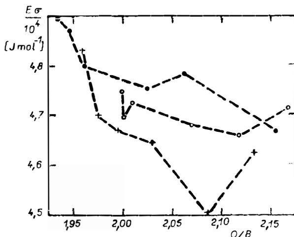
Fig. 7.  $E_a$  vs. the  $\text{O/B}$  ratio in glasses having the composition  $X \text{Li}_2\text{Cl}_2 - Y \text{Li}_2\text{O} - 7 \text{B}_2\text{O}_3$  ( $\bullet$  —  $X = 2$ ;  $+$  —  $X = 2.5$ ;  $\circ$  —  $X = 3$ ).
