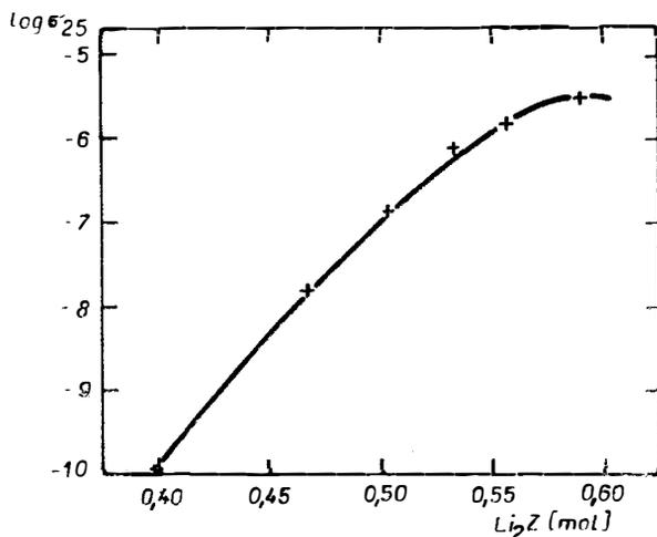
Fig. 4.  $\log \sigma_{25}$  vs.  $\text{Li}_2\text{Z}$  content in glasses having the composition  $X \text{Li}_2\text{Cl}_2\text{—}3 \text{Li}_2\text{O—}7 \text{B}_2\text{O}_3$ .
