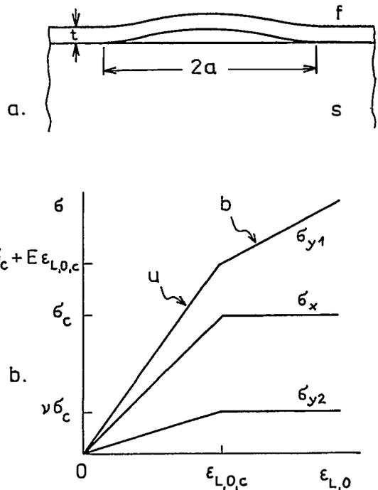
Fig. 2. Buckling of delaminated film due to compressive stresses. a) schematic diagram, b) edge stresses in one-dimensional delamination with a hot spot as a function of local compressive strain  $\epsilon_{L,0}$  in part 1.  $\sigma_c$  - critical stress,  $\epsilon_{L,0,c}$  - critical strain,  $E$  - Young's modulus,  $\nu$  - Poisson's ratio, u, b - unbuckled and buckled state.
