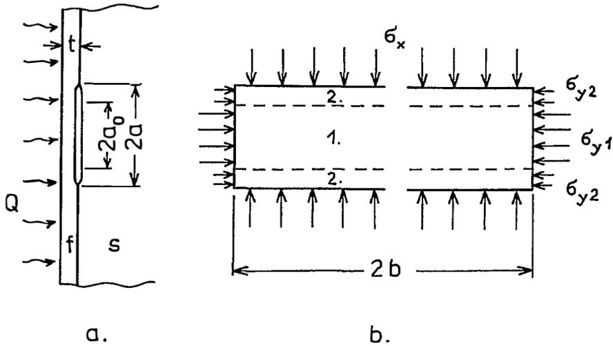
Fig. 1. Delamination with a hot spot. a) schematic diagram, b) stresses in one-dimensional delamination
