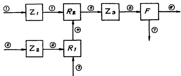
*Fig. 1. Schematic diagram of a neutralizing station. 1 – acid water, 2 – lime, 3 – fresh water, 4 – milk of lime, 5 – neutralization sludge, 6 – waste water, 7 – filter cake,  $Z_1$  – acid water tank,  $Z_2$  – powder lime bin,  $Z_3$  – neutralization sludge tank,  $R_1$  – tank for preparation of milk of lime,  $R_2$  – neutralization reactor, F – filterpress.*
