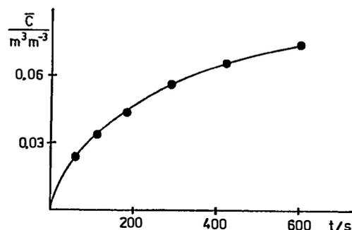
Fig. 4. Experimentally established time dependence of mean concentration of liquid in the gypsum.
