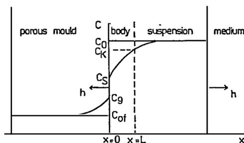
Fig. 1. Schematic representation of body formation and solidification including transmission of liquid through the porous mould.
