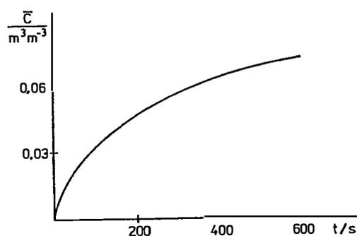
Fig. 6. Calculated time dependence of mean concentration of liquid in the gypsum.
