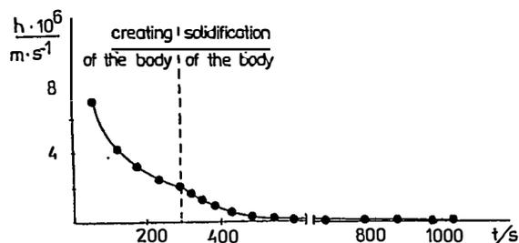
Fig. 2 Time dependence of the surface flow of the liquid.
