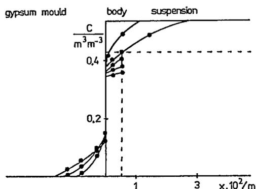
Fig. 3. Experimentally established time development of concentration profiles.
