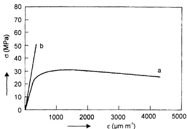
Figure 3. Relative transverse deformations of a) reinforced pastes, b) non-reinforced pastes
