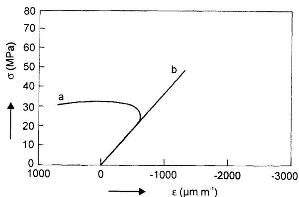
Figure 4. Relative volume deformations of a) reinforced pastes, b) non-reinforced pastes
