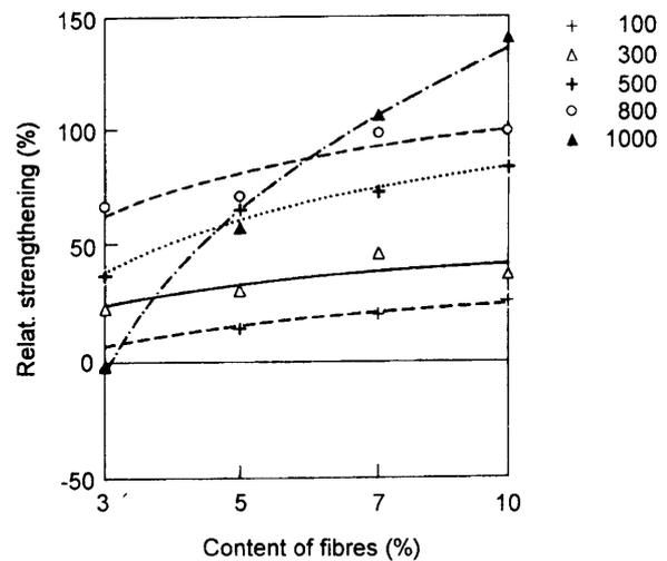
Figure 1. Increase in strength vs. the content of fibres
