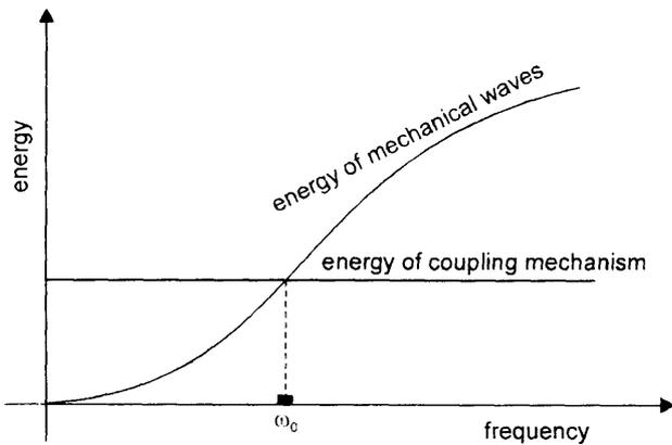
Figure 5. Scheme of relationship between energy of acoustical waves and coupling mechanism energy.
