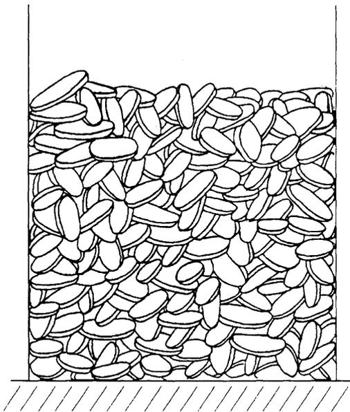
Figure 6. Scheme of  $\text{YBa}_2\text{Cu}_3\text{O}_{7-x}$  powder system, which was not exposed by sound wave propagation. No direction is preferred from the particles orientation point of view.
