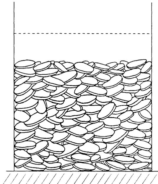
Figure 7. Scheme of  $\text{YBa}_2\text{Cu}_3\text{O}_{7-x}$  powder system exposed by sound wave of "optimal frequency" propagation. Transported energy is equal to energy of coupling mechanism and the spontaneous changes are generated. The changes gradually lead to state of minimal energy. Most powder particles are oriented close to horizontal level in that state.
