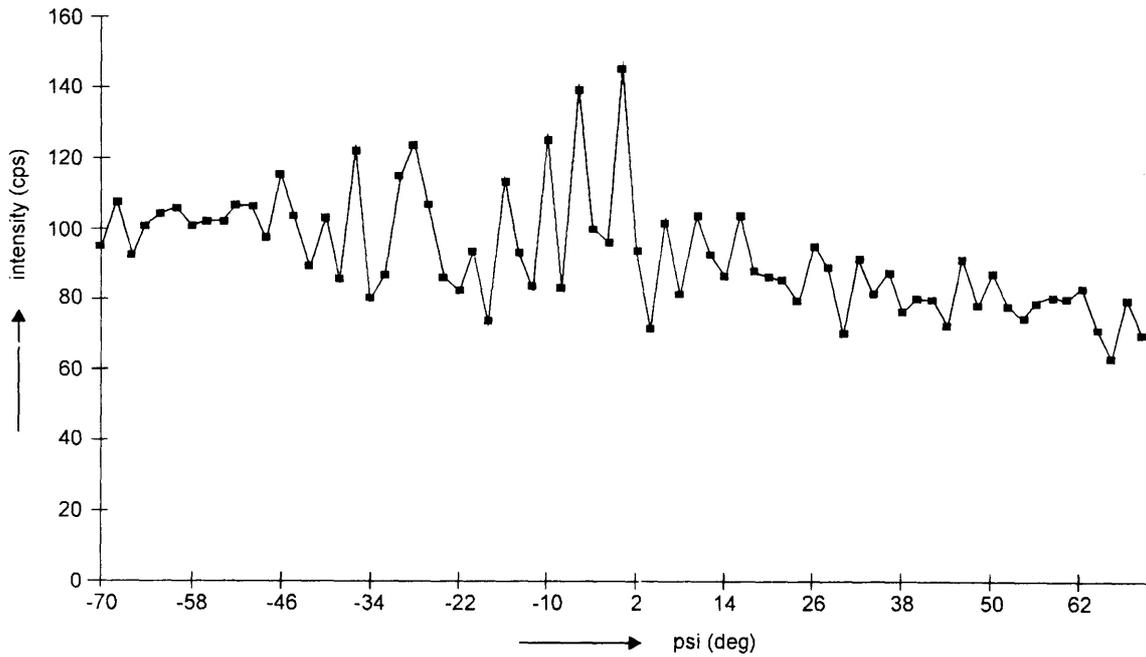
Figure 4. Angular distribution of 002 reflection intensity for the sample prepared from powder exposed by acoustical waves of frequency 1 kHz during time interval 1 hour.
