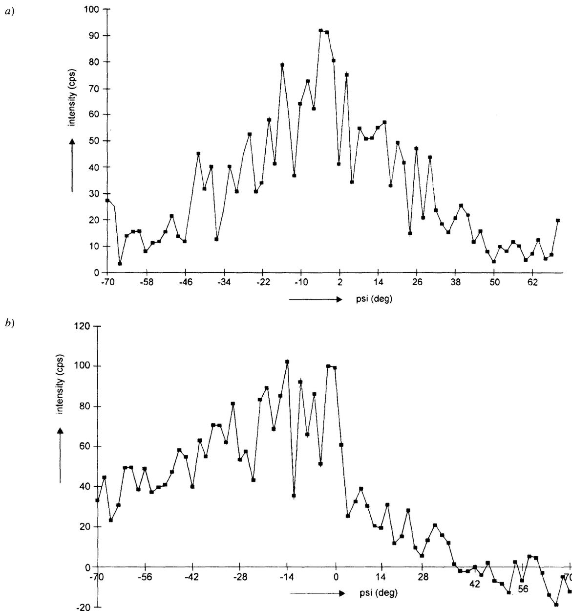
Figure 3. Angular distribution of 002 reflection intensity for the sample prepared from powder exposed by acoustical waves of frequency 500 Hz during time interval 1 hour.
