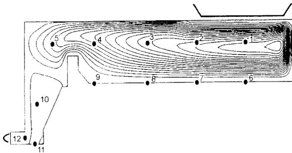
Figure 1. Geometry and flow structure of the TC 21 test case furnace.
