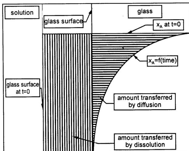
Figure 3. Schematic representation of amount of moveable glass species transferred into the solution.
