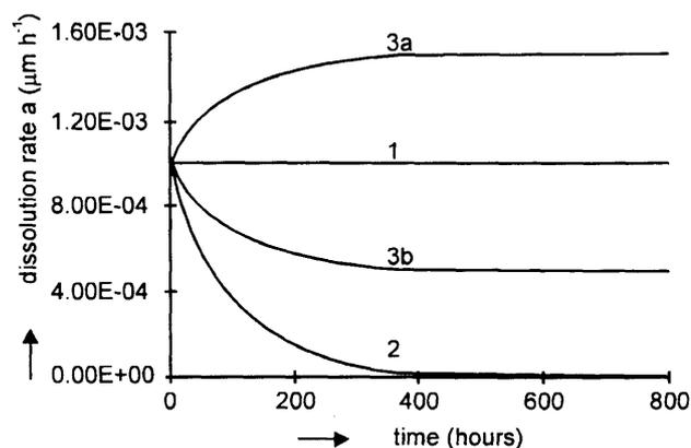
Figure 1. Possible time dependencies of glass dissolution rates. 1 - Constant dissolution rate. ( $D/h \rightarrow \infty$ ,  $F \rightarrow \infty$  and/or  $S/V \rightarrow 0$ ). 2 - Dissolution rate decreases to zero ( $F=0$  and/or  $(D/h)_n \rightarrow 0$ ). 3 - General time dependence of glass dissolution rate according to equation (1) a)  $a_n > a_0$ ; b)  $a_n < a_0$ .
