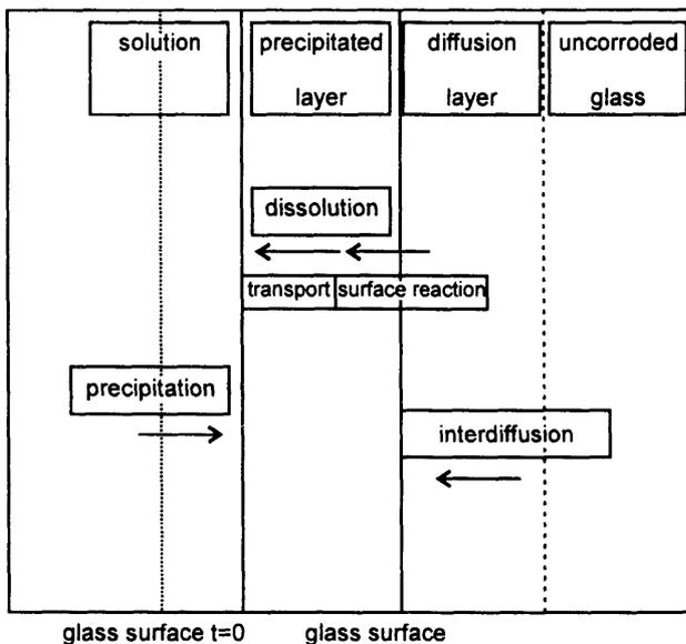
Figure 2. Schematic representation of processes involved in glass dissolution.
