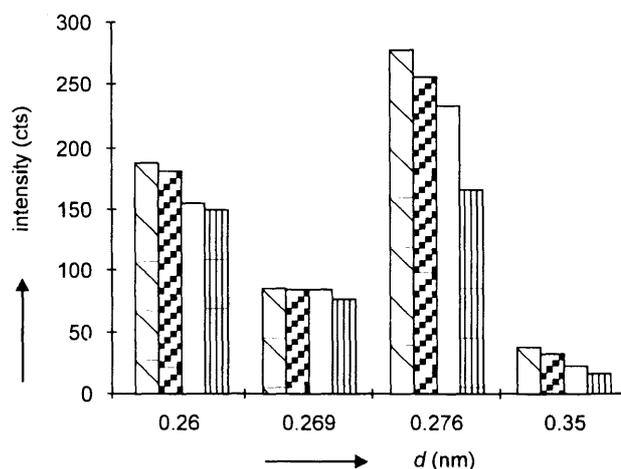
Figure 1. The integral intensities of diffraction lines characteristics for clinker minerals for starting sample and the same sample after treatment in different mills.
