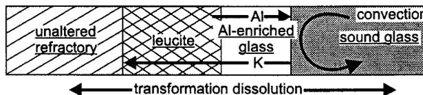
Figure 1. Wear of a refractory pot (section).
