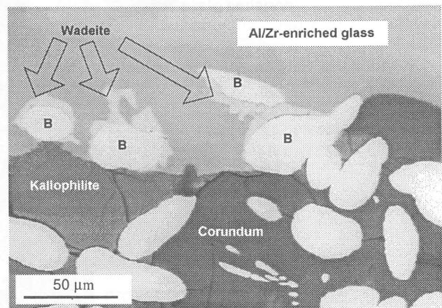
Figure 8. Section through an ER 1711 block in the melting area showing small crystals of wadeite - SEM, polished section, backscattered electron image.
