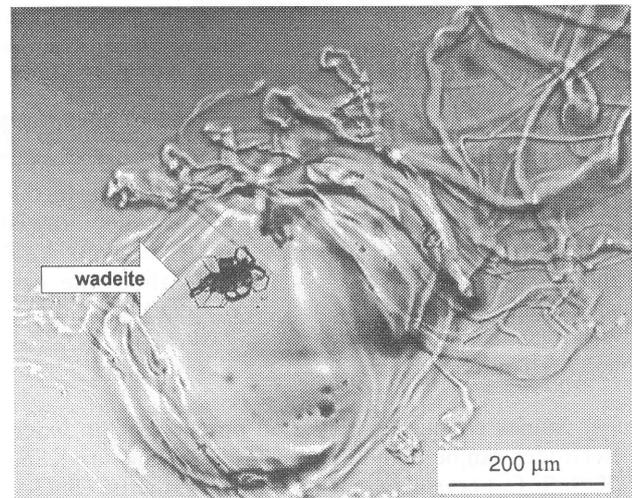
Figure 7. typical vitreous knot containing crystals of wadeite - PLM
