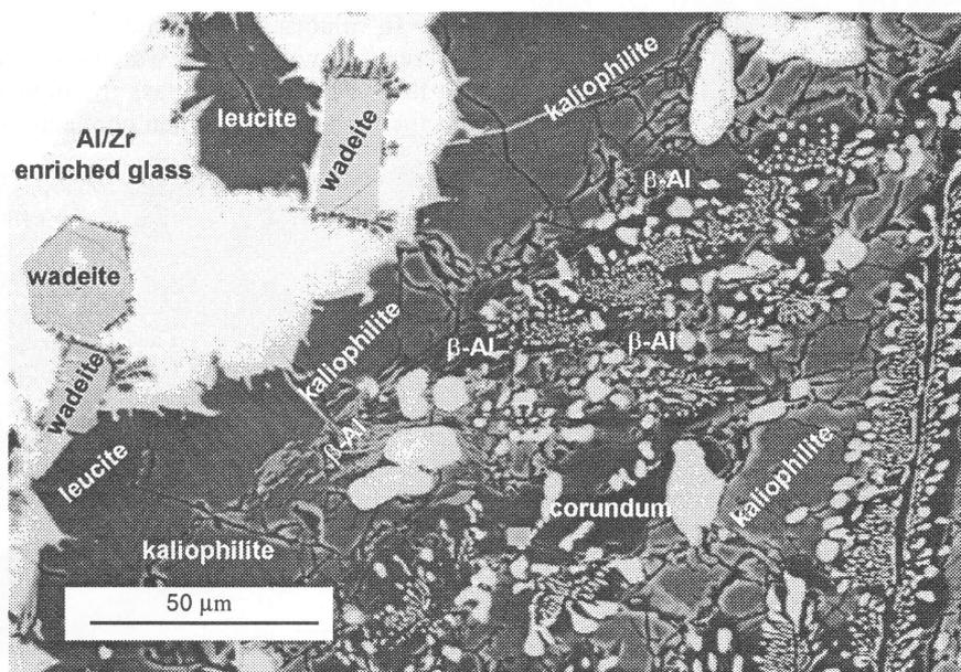
Figure 9. Section through an ER 1711 block in the melting area - crack showing crystals of wadeite - SEM, polished section, backscattered electron image.
