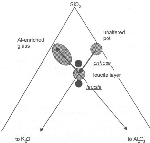
Figure 2. Pot corrosion : evolution of the ternary compositions (example with a 20% Al<sub>2</sub>O<sub>3</sub> pot clay).
