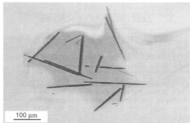
Figure 5. Hexagonal eskolaite platelets (black) in an aluminous solution sac (dark grey) - SEM, polished section, backscattered electron image.
