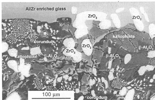
Figure 6. Section through a worn ER 1711 electrode block in the drilling corrosion area - SEM, polished section, backscattered electron image.
