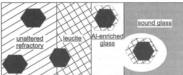
Figure 3. Mechanism of formation of grog particles stones (grog particles painted black).
