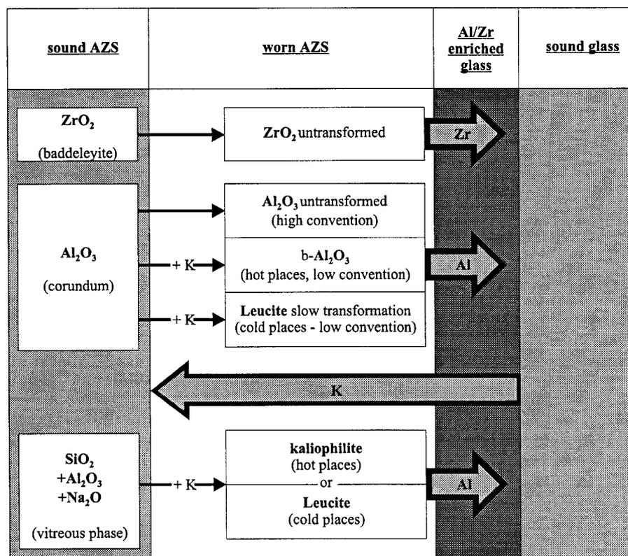
The composition of the phases present in stones allows to trace them back to their source : kaliophilite in a worn AZS stone will show that it comes from the melting area. Beta-alumina in a worn AZS stone and / or wadeite in solution sacs will show that it comes from places with low convection currents.
