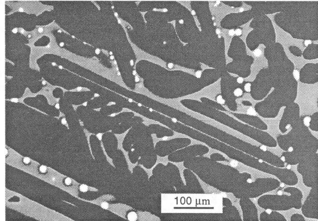
Figure 4. Dendrites of leucite (black) and droplets of the phase rich in Pb, As (white), SEM, polished section, backscattered electron image.
