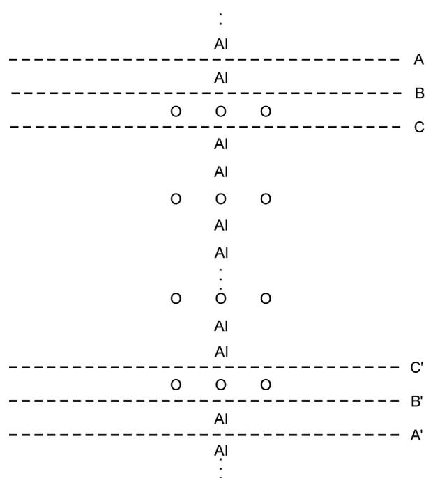
Figure 1. Arrangement of atomic (001)-planes schematically projected on the  $c$ -axis.
