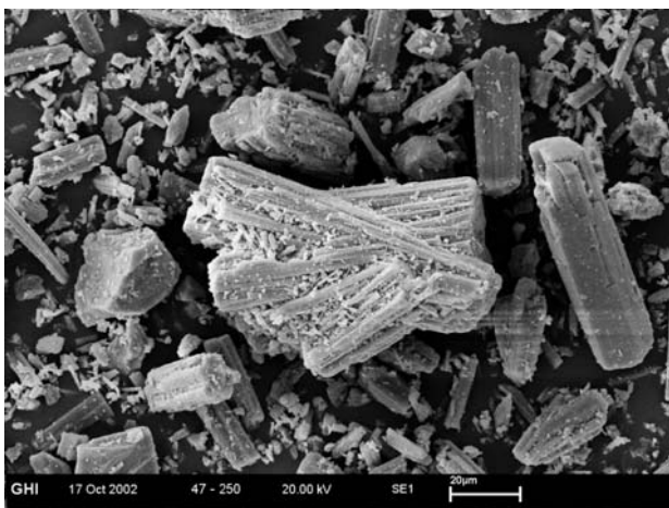
Figure 4. SEM micrograph of medical gypsum: loss on ignition = 6.88 %.
