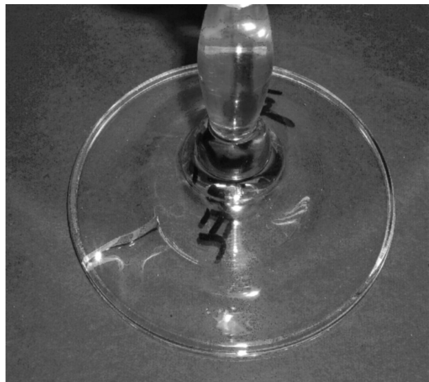
Figure 7. Detail of a real stem bottom from production with a radial crack (in a white circle)
