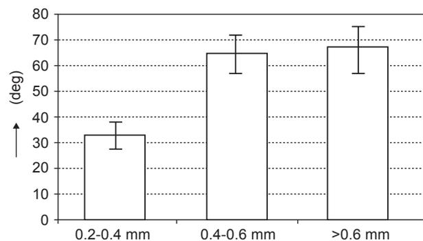
Figure 3. Advancing contact angles of composite samples (R-glass + M130) with different open pores (sizes: 0.2-0.4 mm, 0.4-0.6 mm, >0.6 mm).
