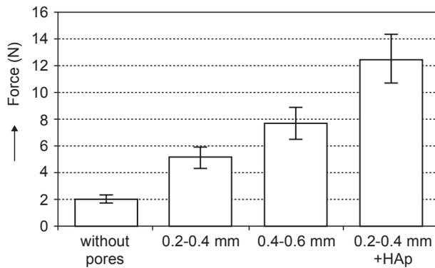
Figure 6. Results of R-glass + M130 and R-glass + M130 + HAp pull-off tests.
