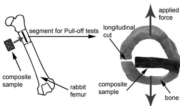
Figure 2. The measured sample for pull-off tests (based on Nakamura et al. [25, 27]).
