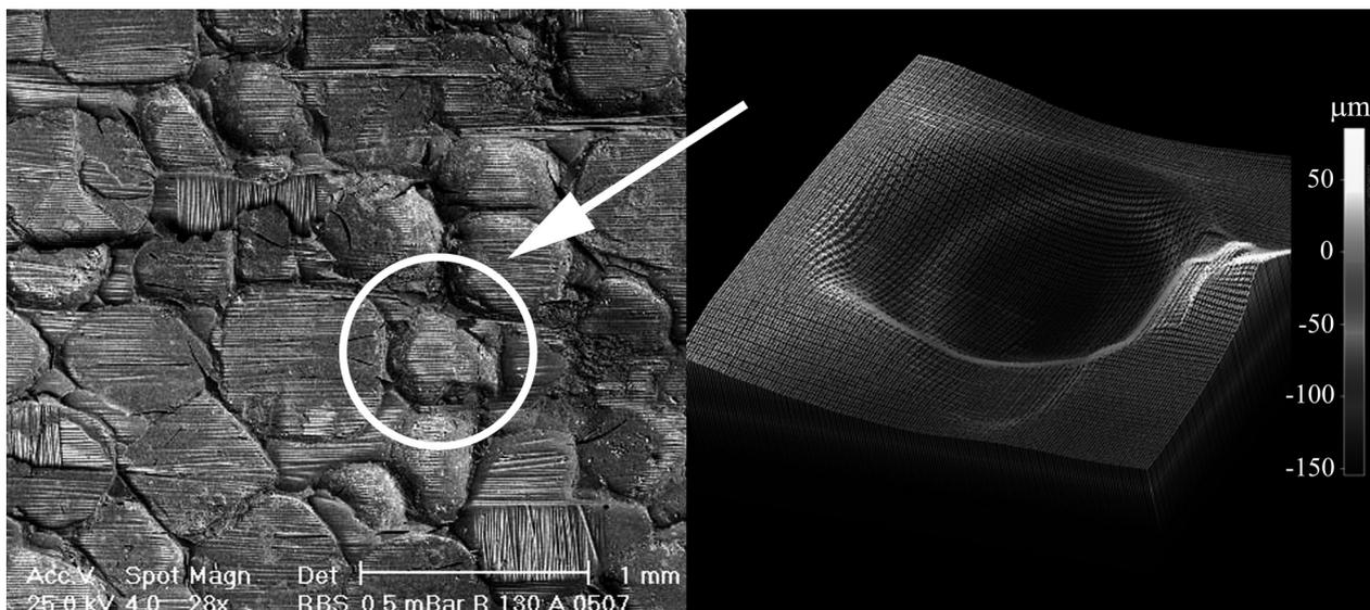
Figure 1. Surface and pore (right) structure of a composite with a modified surface (open pores 0.4-0.6 mm).
