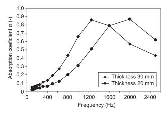
Figure 2. Absorption coefficient of geopolymer/sand mixture Geo 2 (fractions of quartz sand 0.3-0.6 mm and 0.6-1.2 mm).
