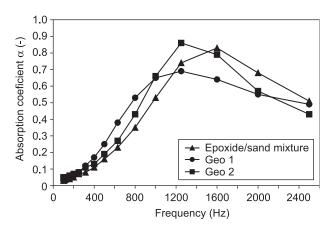
Figure 3. Overview of Geo 1, Geo 2 and epoxide/sand mixture results of absorption coefficient (thickness of 30 mm).
