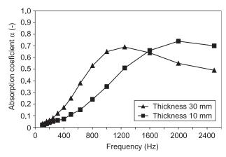
Figure 1. Absorption coefficient of geopolymer/sand mixture Geo 1 (fraction of quartz sand 0.3-0.6 mm).
