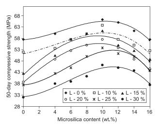
Figure 3. 50-day compressive strength of cement pastes containing different proportions of microsilica and limestone powder.
