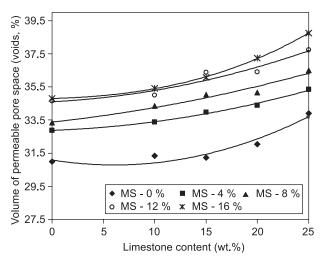
Figure 4. Volume of permeable space of cement pastes containing different proportions of microsilica and limestone powder.
