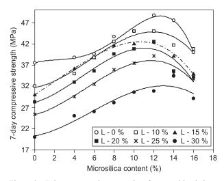
Figure 2. 7-day compressive strengths of ternary blended cements with limestone powder and microsilica.
