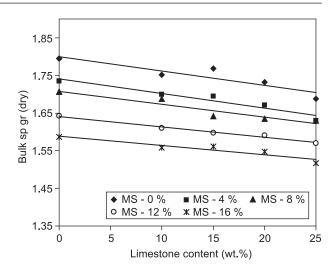
Figure 5. Bulk specific gravity of cement pastes containing different proportions of microsilica and limestone powder.
