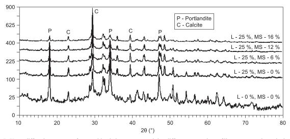
Figure 7. X-ray diffraction patterns of ternary blended cements containing different proportions of limestone powder and microsilica after 28 days of hydration.
