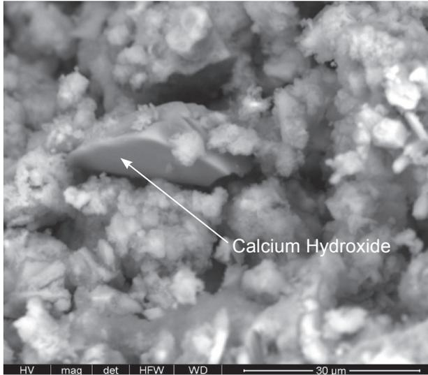
having a sharp portlandite peak at that age. The EDX analysis confirms the presence of honeycomb CSH (II) that contains high calcium content than the silica. After 7 days, the micrograph indicates the growth of hydration products with the increase of ill-crystallized CSH phases and hexagonal crystals of  $\text{Ca}(\text{OH})_2$  as well as little plates of Friedel's salt that appear within the matrix Figure 7b.
